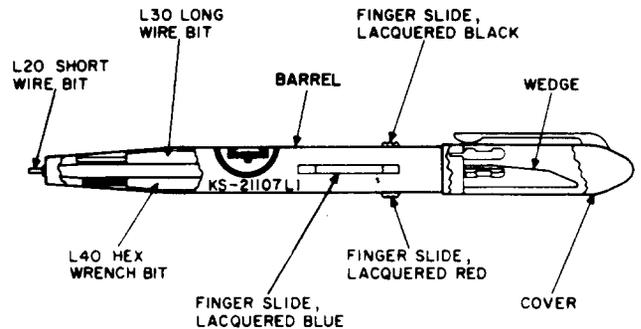
Consists of a brass, double-ended, pen-type combination tool containing three retractable bits at one end and a wedge-shaped extension at the other end.
