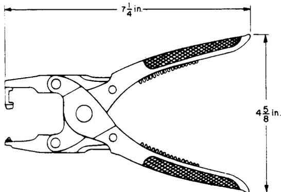
Pawl pin replacer. Forms part of the 1001A tool kit. For use in replacing pawl pins on 197- and 198-type switches.
