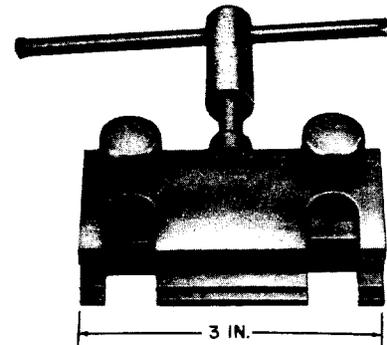
Core plate replacer. Order this tool for replacement purposes only if the office is equipped with the 1012A tool kit. The 1012A tool kit is no longer available as a complete kit. For use in replacing core plates of 286-, 287-, and 288-type relays.
