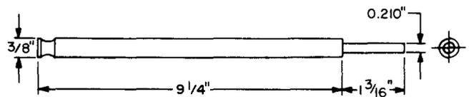
Torque rod. For use in checking the tension of the clutch idler spring on the KS-13834 perforator.
