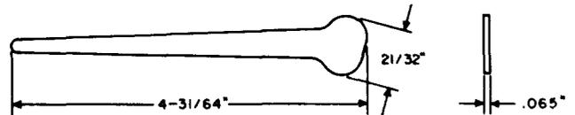
Stirring rod. For use in stirring paint and filling the 463A and 464A tools with paint in multiple marking work.
