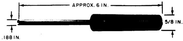
Female screwdriver. For use in adjusting the 1548-type inductors of the 486-type networks in ANI identifier frame.
