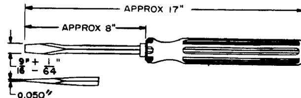
Replaces the T handle screwdriver R-58442 and the AT-6860 double grip screwdriver. For use primarily on clutches in panel central offices.
