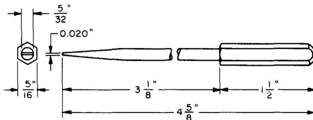
A 3-1/8 inch screwdriver. Replacement part for the 72 tool. For use on reciprocating bar-type interrupters and connecting blocks.
