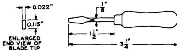
For use on the 51-type dial testers, Palmer master switches, and emergency lighting relays.
