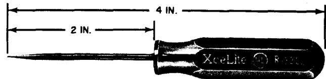
For use in adjusting potentiometers of group pilot insert units of L-Multiplex equipment.
