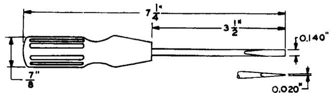
Replaces the 35 tool. Forms a component part of the 221 tool used in the maintenance of central office apparatus.
