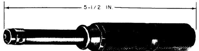
Screwdriver is set for 5 ounce-inches of torque. For use in tightening U-type relay mounting screws equipped with grommets. Screwdriver bit must be ordered separately for use with this tool. Refer to Section 074-205-114 for screwdriver bit used with this tool.
