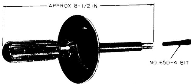
Equipped with 650-4 bit only. A torque screwdriver having a capacity of 12 inch-pounds. For use in tightening mounting screws of wire spring type relays equipped with P-19A890 flexible mountings.
