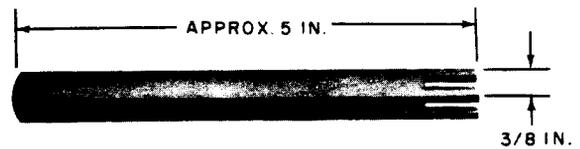
Coil setter. Replaces the 717A tool. Forms part of 1014B tool kit. For use in replacing coils of AF-, AG-, AJ-, AK-, 286-, 287-, and 288-type relays.
