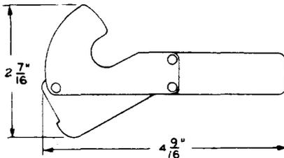
"A" cam short circuiting tool. Replaces the 218 tool. For use on A- and B-type sequence switches and 155A and 157-type interrupters.
