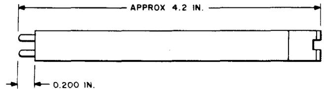
**Shorting clip.** For use when installing and removing shorting clip in the No. 1 Electronic Switching System.
