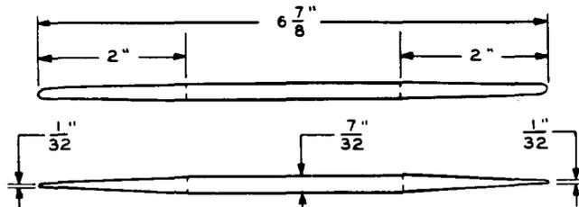
Primarily used in panel offices for testing commutator spring tensions. A wire position tool and other general uses.
