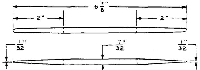
Primarily used in panel offices for testing commutator spring tensions. A wire position tool and other general use. **DO NOT USE FOR SOLDERING OPERATIONS.**
