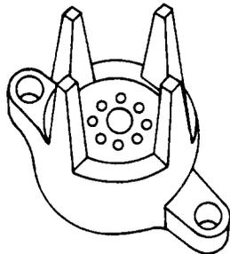
The JE13 tube pin straightener is for use on seven-pin miniature vacuum tubes.
