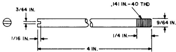
Threaded stud. For use in reassembling bearings of small motors and generators.
