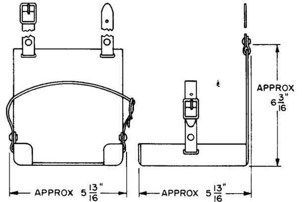
Metal tray for carrying Sensitive Research Instrument Corp. Model "Bellud" millivoltmeters and Weston Model 931 voltmeters while taking battery readings. Equipped with leather straps for fastening around the neck and for securing the meter to the tray.
