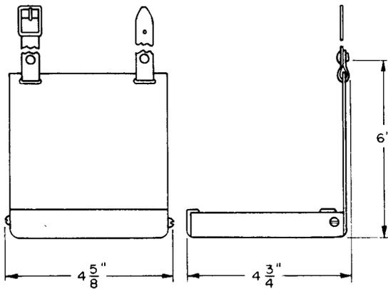
Metal carrying tray for carrying a Weston Model 280 or 281 voltmeter while taking battery readings. Equipped with leather strap for fastening around the neck.
