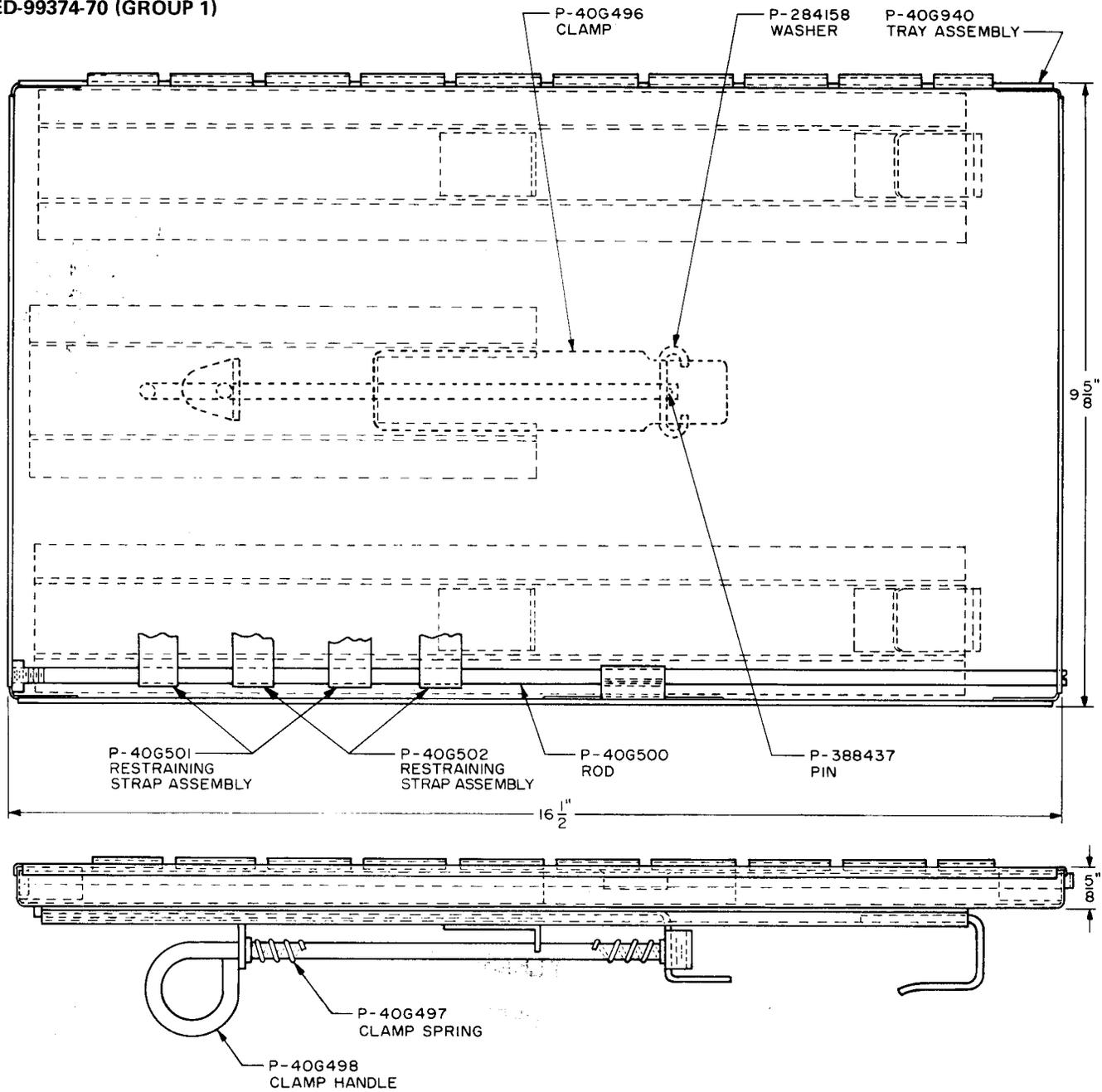
Instrument tray. Designed to hold a variety of ammeters, ohmmeters, and voltmeters used in central offices.
