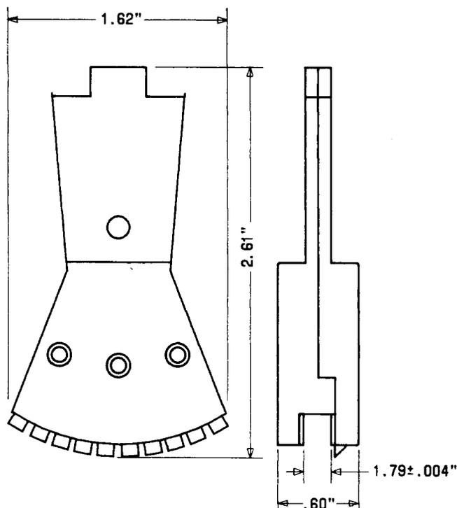
Used With a 788A1 Handle for trimming off unused portions of conductors installed on an 88-type wiring block.
