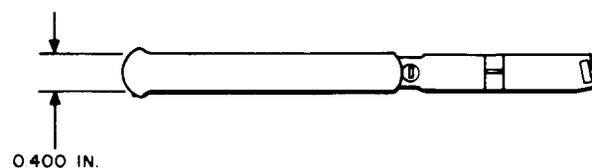
**A Hand Operated Punch With Insulated Handles.** It is intended for use in central offices to remove damaged Mylar from step-by-step banks.
