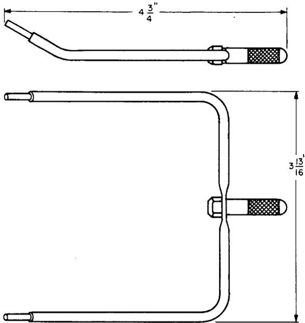
For use in tuning microwave cavities in the TD-2
