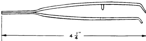
Replaces the D-170283 tweezers. For use in replacing cards on 304- and similar-type switches.
