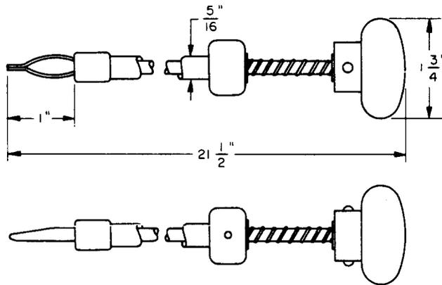
Spring tweezers. Replaces the 77 tool. For use in holding wires to jack terminals while soldering.
