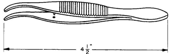
4-1/2 inch bent tweezers. Part of the 1004A tool kit. Replaces the R-2217 tweezers. For use on relays and KS-13834 perforators.
