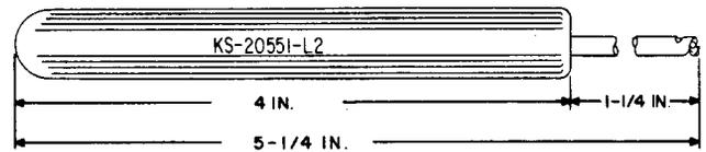
A manually operated wire-unwrapper tool used for removing wire from terminals having solderless-wrapped connections on the AMA translator frame and in areas of extreme wire congestion. Will accommodate terminals with cross-section dimensions up to 0.032 by 0.062 inches or with diagonal dimensions up to 0.070 inches.
