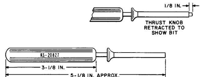
A manually operated wire-unwrapper tool, with an insulated retractable sleeve, used primarily to unwrap and remove solderless-wrapped connections of 22-, 24-, and 26-gauge wires. Replaces the KS-16492 L2 wire-unwrapper.
