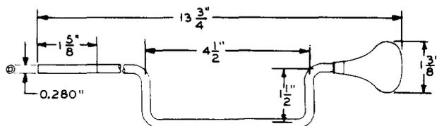
Includes the 27 key pipe. For use in winding Model 6 Calculagraphs.
