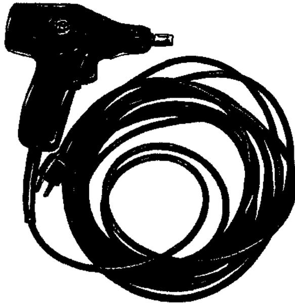
The KS-21232 L1 (electric) wire wrapping gun is used for 20-gauge through 30-gauge wire. It is a lightweight pistol shaped, double insulated, 115-volt ac powered gun with a 20-foot cord. A low transient voltage output permits its use on or near "live" equipment, including ESS. Bits and sleeves currently standardized for 22-, 24- and 26-gauge wire may be used in this gun. Bits and sleeves for 28- and 30-gauge wire are available commercially as indicated below:
