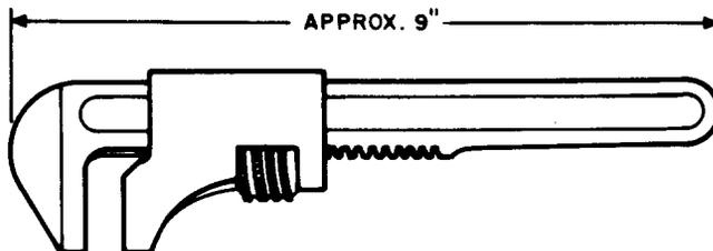
A 9-inch adjustable auto or thin monkey-type wrench. Maximum opening is 2-5/8 inches. Replaces the No. 9, Model G, Billings and Spencer wrench. For use on AMA KS-13928 cleaning cabinet.
