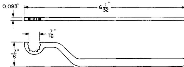
A 7/16-inch open offset box wrench. For use on the KS-13834 perforators.
