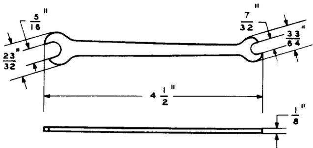
A 5/16-inch and 7/32-inch open double-end flat wrench. Replaces the 7/32-inch and 5/16-inch ends of AECO H-7062 and H-7063 hex. open-end flat wrenches. For general use.
