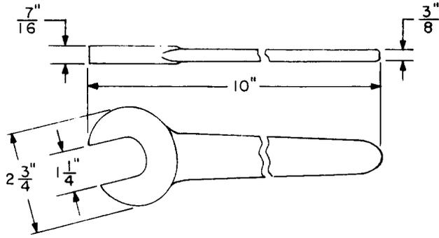
A 1-1/4 inch open single-end flat wrench. For use on friction roll drives, vertical drive shafts, and for general use in power equipment.
