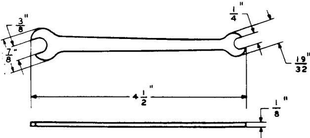
A 1/4-inch and 3/8-inch open double-end flat wrench. Replaces the 244 and 306 tools and the 1/4-inch and 3/8-inch ends of AECO H-7062, H-7063, and H-42316 hex. open-end flat wrenches. For general use.
