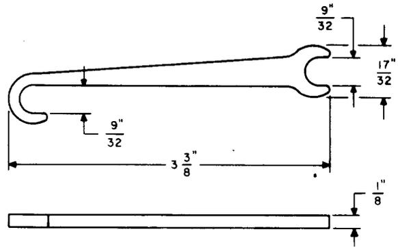
A 9/32-inch open double-end flat wrench. For use on clutch adjusting nuts.
