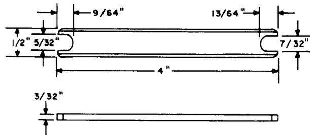
A 5/32-inch and 7/32-inch open double-end flat wrench. Replaces the 75 tool. For general use.
