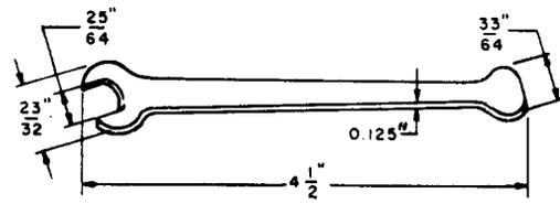
A 25/64-inch flat open-end wrench. For use on the 197- and 198-type switches.
