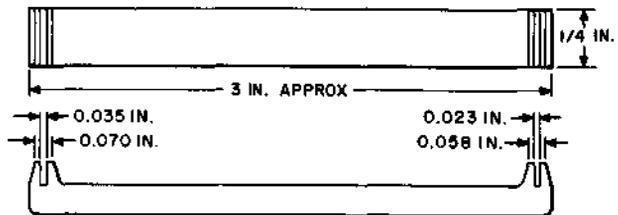
For use in adjusting normal post springs on 197-type switches.
