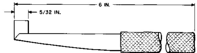
For use on sequence switches and 157-type interrupters.
