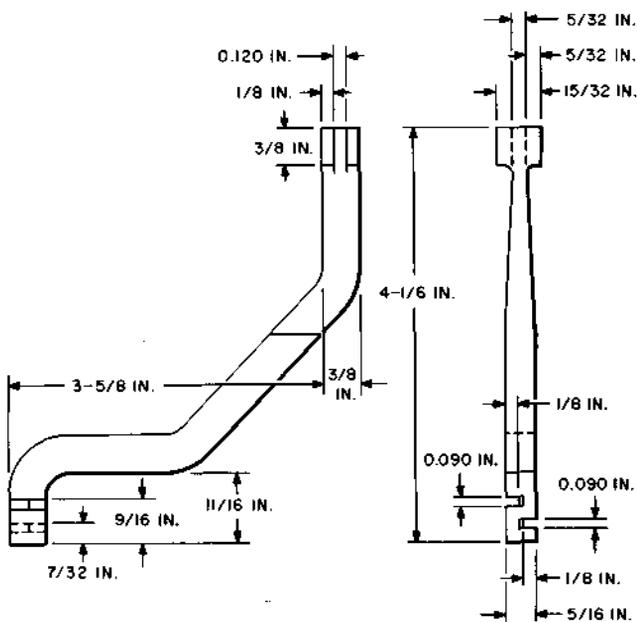
For use on 200-, 206-, 209-, and 211-type selectors, 25-point rotary switches, and 1-type translators.
