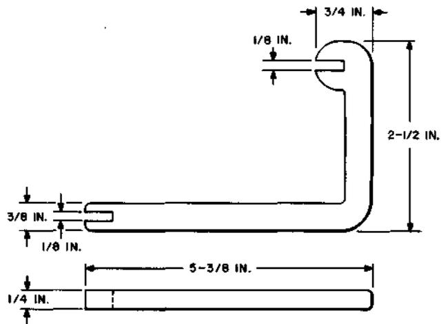
Replaces the AECo H-7056 armature adjuster. For use on 197- and 198-type switches.
