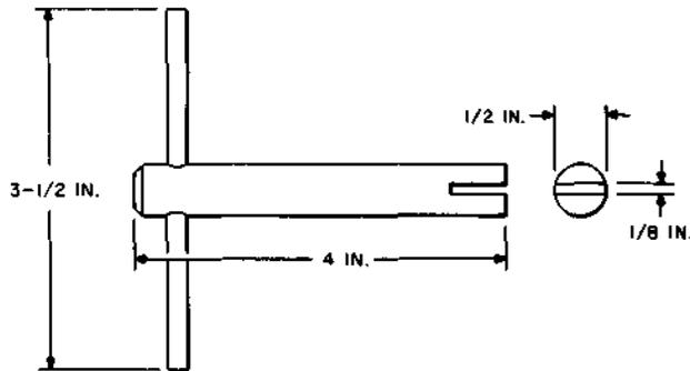
For use on plunger-type line and out-trunk switches.
