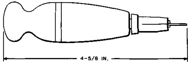
Six needles are furnished with each tool. For use on panel elevator apparatus.
