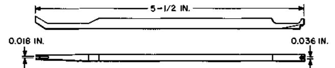
For adjusting cover spring on AF-, AG-, AJ-, and AK-type relays.
