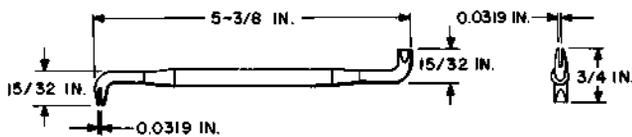
For use on step-by-step type relays and 197-, 198-type switches.
