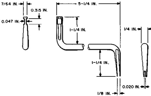
Similar to the 380A tool except that the openings shown at left in the above illustration are wider. For use on panel multiple brushes in cases where the 380A tool cannot be used because of brush springs being too wide.
