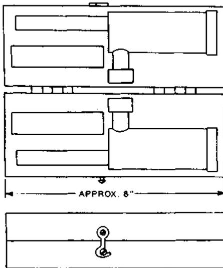
A black finished wooden case with a hinged cover held closed by a latch. Part of the No. 1003A tool kit and used for housing the tools of that kit.
