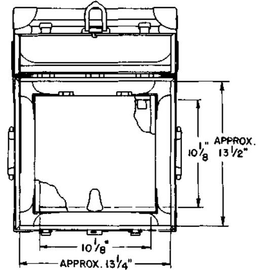
Consists of an inner case in an outer case with shock absorbent padding between the cases. Both cases have wood frames covered with black vulcanized fibre, and hinged lids. The key to the lock on the outside lid of all KS-14131 Carrying Cases, now manufactured, is the same as that used KS-14253 Carrying Cases.
