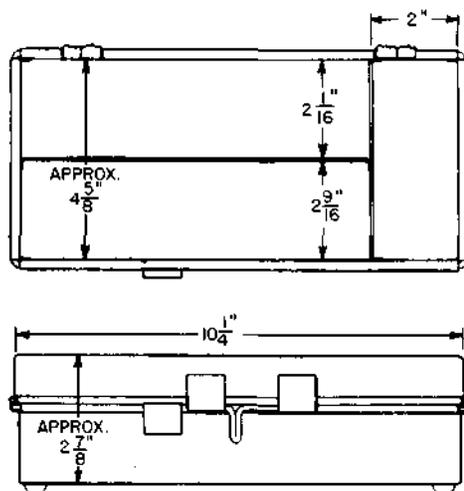
A black finished sheet metal case with a hinged cover held closed by a latch. The interior is divided into 3 compartments.
