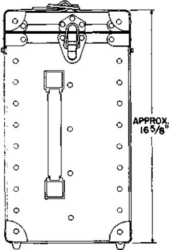
Consists of a vulcanized fibre covered wooden case having a carrying handle and a removable cover. A KS-16157-L1 Strap is provided. The carrying case is part of the No. 1004B tool kit and is used for housing the tools of that kit.
