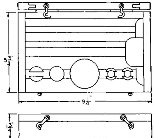
A black finished wooden case with a hinge cover held closed by a latch. Part of the No. 1000A tool kit and used for housing the tools of that kit.
