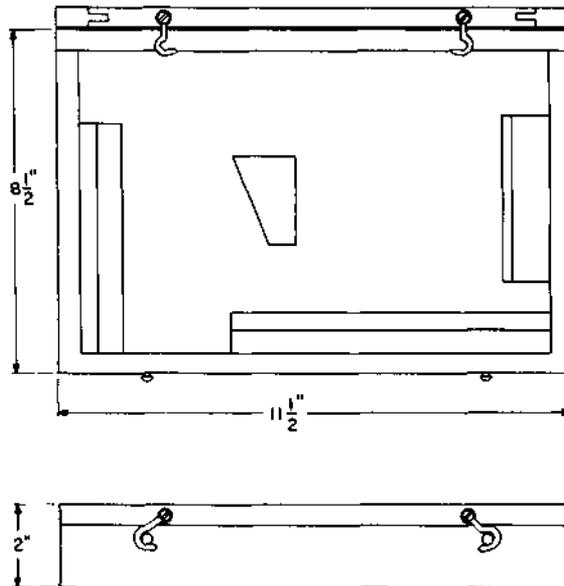
A gray finished wooden case with a hinged cover held closed by a latch. Part of the No. 1014A tool kit and used for housing the tools of that kit.
