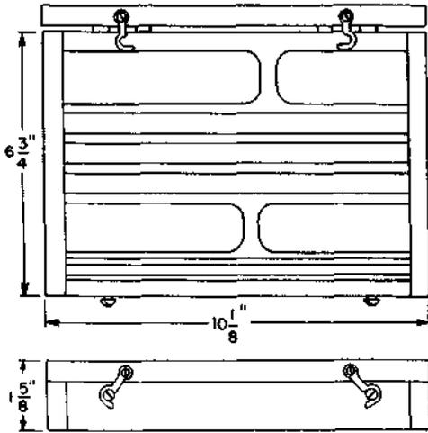
A black finished wooden case with a hinged cover held closed by a latch. Part of the No. 1002A tool kit and used for housing the tools of that kit.
