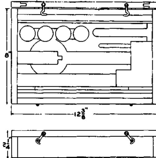
A gray finished wooden case with a hinged cover held closed by a latch. Part of the No. 1012A tool kit and used for housing the tools of that kit.
