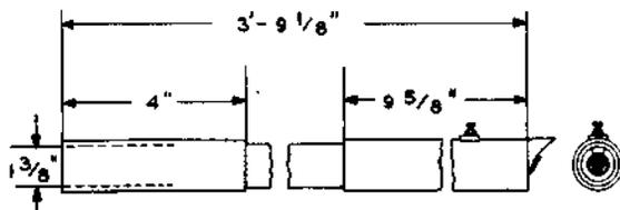
Consists of a fiber tube nozzle and a 3 foot long flexible hose. Furnished with one KS-3093 brush.
