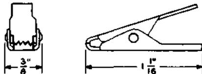
For general use on test cords when the clip is to be soldered to the cord. The jaws can be insulated by means of a 108 cord tip (insulating tubing).
