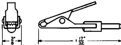
For general use on 360A, B, and C tools. The jaws can be insulated by means of a 108 cord tip (insulating tubing).
