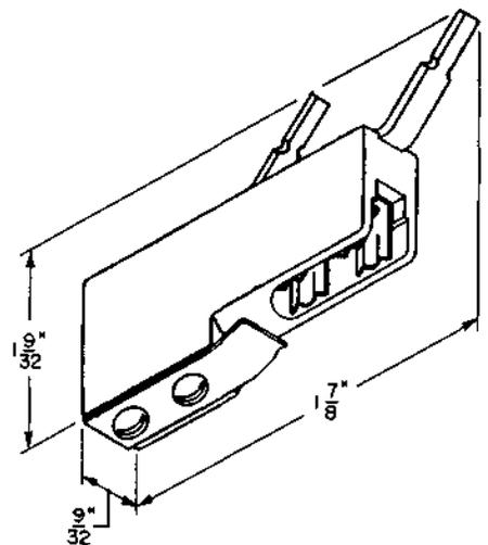
For use on 121-type protectors and 300-type connectors to provide means for connecting to the cable pairs at the test terminals. This clip may be used with the M2EM cord for bypassing the protector.
