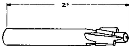
For use in replacing springs and studs of Dzus fasteners.
