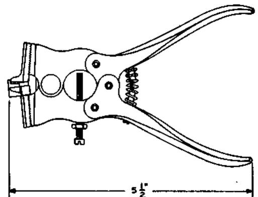
For cutting slots in straps to separate groups, when required, on 15-type banks.
