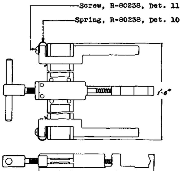
For use on vertical drive shafts and associated apparatus.
