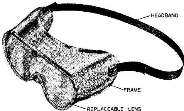
These goggles can be worn over spectacles. The lenses are impact resistant, the frames are ventilated and the headband is adjustable.
