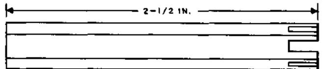
For use in removing rivets of Dzus fasteners.
