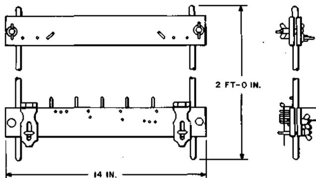
For use in connecting conductors at terminal strips.
