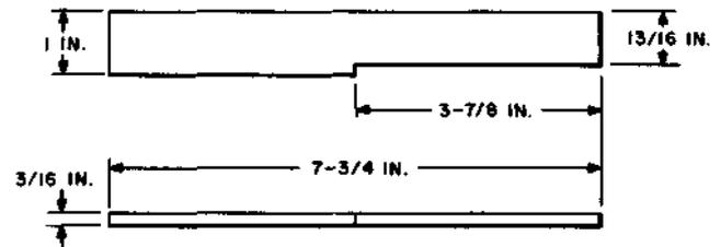
For use in replacing worn contact springs of sequence switches.
