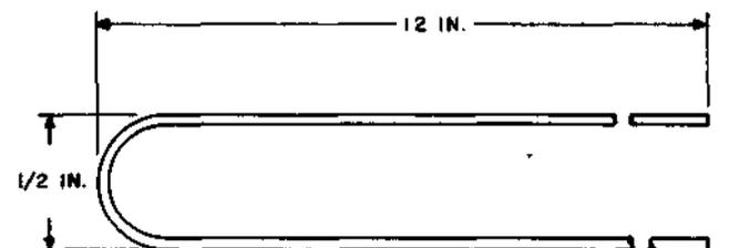
Used as an aid for replacing defective hairpin select wires with the vertical units of a small crossbar switch mounted in an equipment frame.
