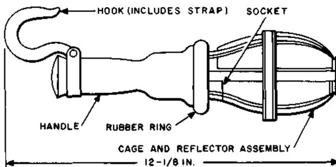
Consists of a soft rubber handle with a fiber guard, a lamp socket and a hook.
