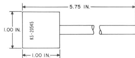
An insulated tool consisting of a rectangular block which is beveled and slotted at one end, and assembled to a rod shape handle at the opposite end. The slot is arranged to accommodate a sheet of KS-7187 cleaning paper.
