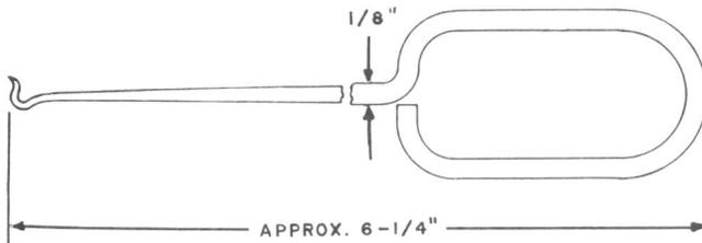
For use in attaching selector elevator apparatus trip rod rotating lever retractile springs and on No. 1A regenerator units.
