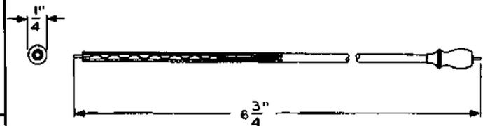
For use with the 486A tool when oiling KS-13834 perforators.
