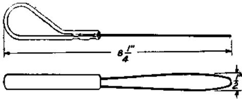
For use in sewing cable (PEX installation only)
