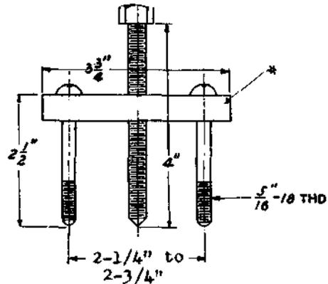
\*Bar slotted to provide differences in center spacing of screws.
