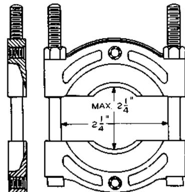
For use with No. 1002 Bearing Puller in removing bearings which cannot be gripped satisfactorily by the puller jaws.
