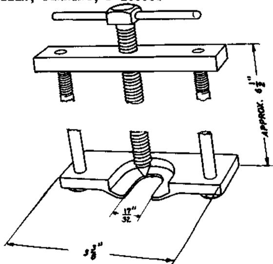
For replacing bearings in KS-7664 and KS-7781 controllers.
