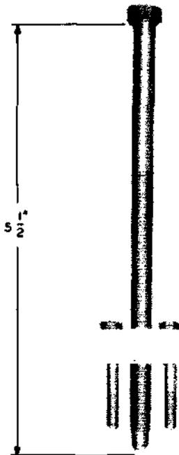
For use with Owatonna Tool Co. No. 950 Bearing Pulling Attachment to remove ball bearing race from shaft of blower motor used in the KS-16001 Dehydrator.
