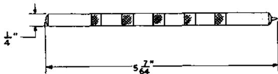
For use in punching knockouts from the KS-14513 cards used in coding the No. 200A blanks for 1-type translators.
