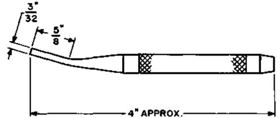
For use in removing the pin holding the shaft bushing of 149-, 152-, 160- and similar type interrupters.
