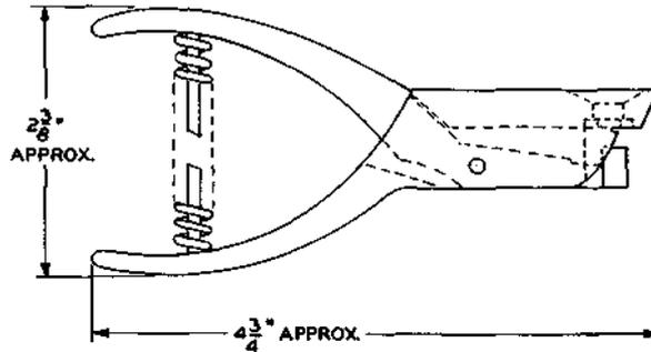
For use in cutting a V-notch in the KS-14513 cards used in coding the No. 200A blanks for 1-type translators.
