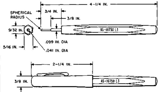
Consists of a metal pin mounted in a cast resin handle and a removable cap.
