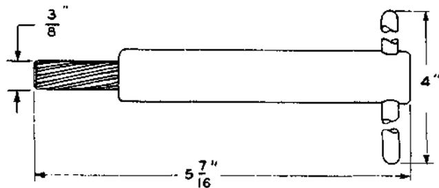
For use with the D-97086 guide and clamp nut, for reaming housing assembly bearings of friction roll drives to relieve overheating.
