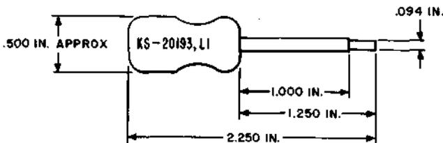
For use in adjusting the regulating repeaters of L4 Coaxial System.
