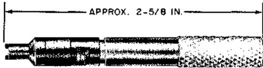
For use in replacing sleeves of 510, 511, and 512 jacks of 608-type switchboards.
