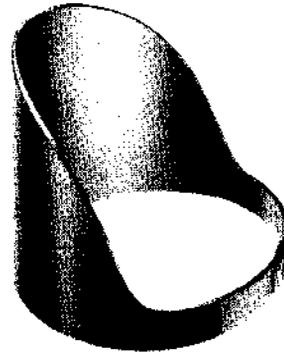
For use in pouring contact protectant compound into the applicator tools used for treating tip- and ring-panel bank terminals.
