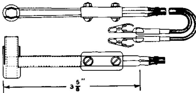
Consists of a 38A lamp socket equipped with an M2CP cord (6' 6"). Intended for use with a 2-type switchboard lamp. The 2-type lamp must be ordered separately.
