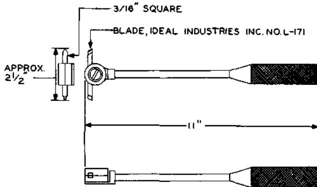
For use on generator and motor commutators and on interrupter drums.
