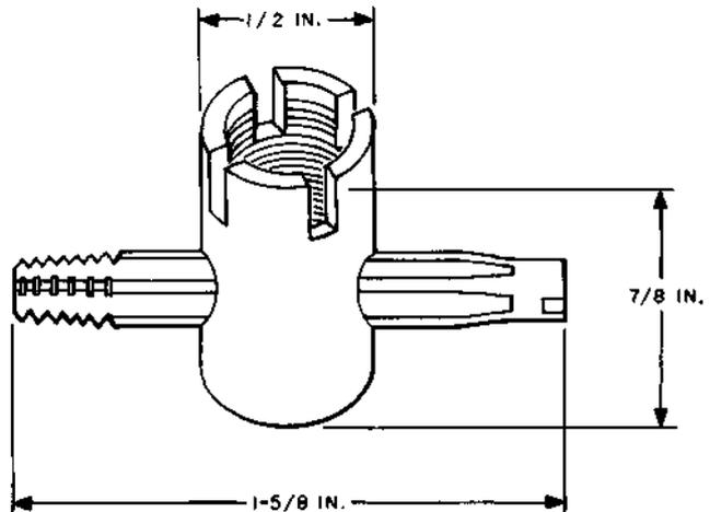
For pressure testing purposes, (Spec. AT-7471 X)
