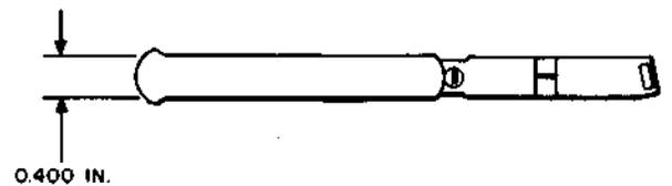
A hand operated punch with insulated handles. It is intended for use in central offices to remove damaged Mylar from step by step banks.
