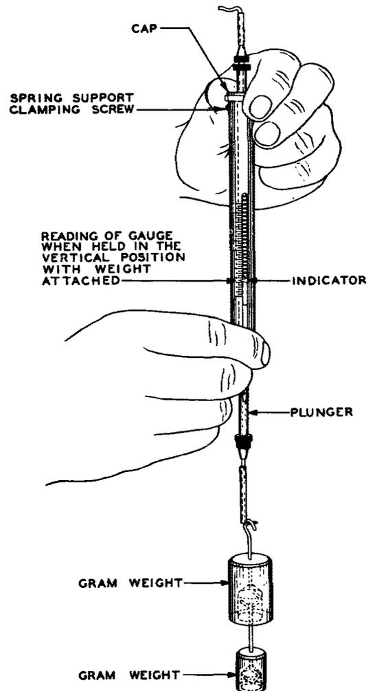
Fig. 8 - Method of Checking Accuracy of a Coil-type Gauge
