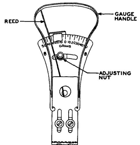
Fig. 10 - Designation of Parts of No. 70G Gauge
