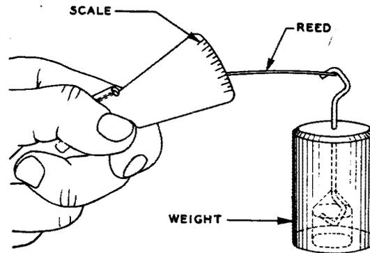
Fig. 5 - Method of Checking Accuracy of No. 62B Gauge
