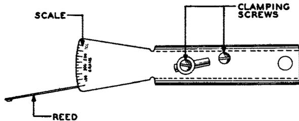
**Fig. 13 - Designation of Parts of No. 62 Gauge**
