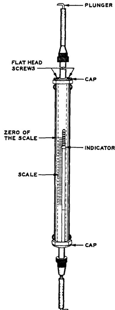
Fig. 16 - Designation of Parts of No. 79A Gauge
