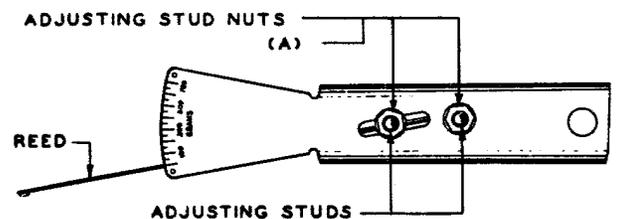
Fig. 3 - Designation of Parts of 62-type Gauge
