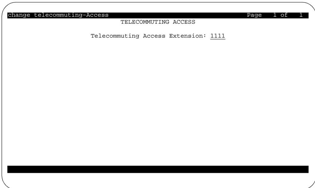
2. In the **Telecommuting Access Number** field, type an extension in accordance with the Dial Plan; for example, **1111**. This is the Avaya EC500 Access Number you provide for users to enable or disable EC500, or to change their Station Security Code. The Telecommuting Access Number must be a direct inward dialing (DID) or a central office (CO) trunk destination for off-premises features to work.
