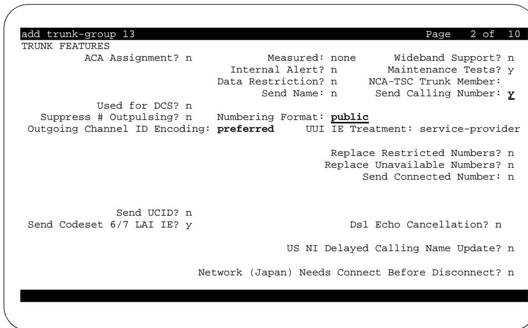
7. Enter the values shown above in the fields **Send Calling Number**, **Numbering Format**, and **Outgoing Channel ID Encoding**.
