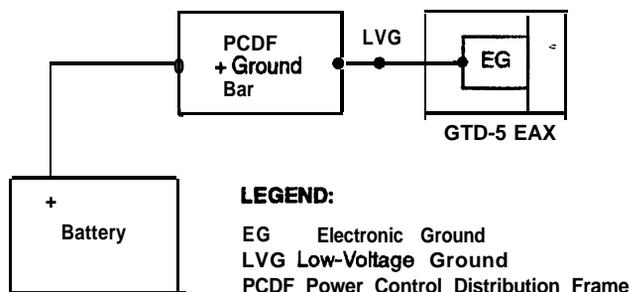
**Figure 5. LVG for PCDF and Co-located PDUFs (Single Bus Only)**
