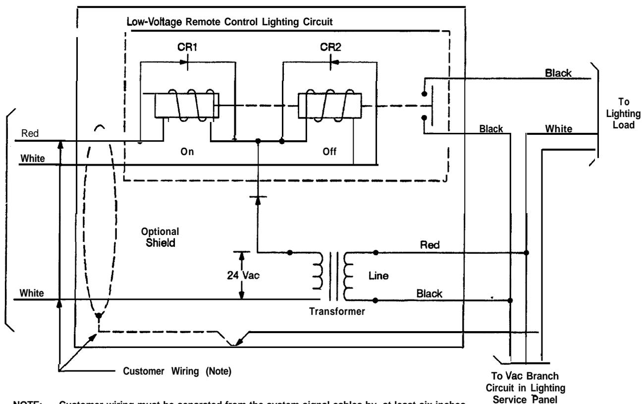
**Figure 1. Typical Low-Voltage Remote Control Lighting Circuit**
