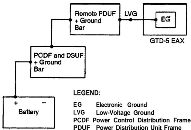
**Figure 6. LVG Arrangement for Single Remote PDUF**
