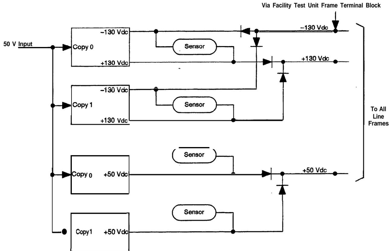
Figure 10. Coin and Pad Disable Batteries
