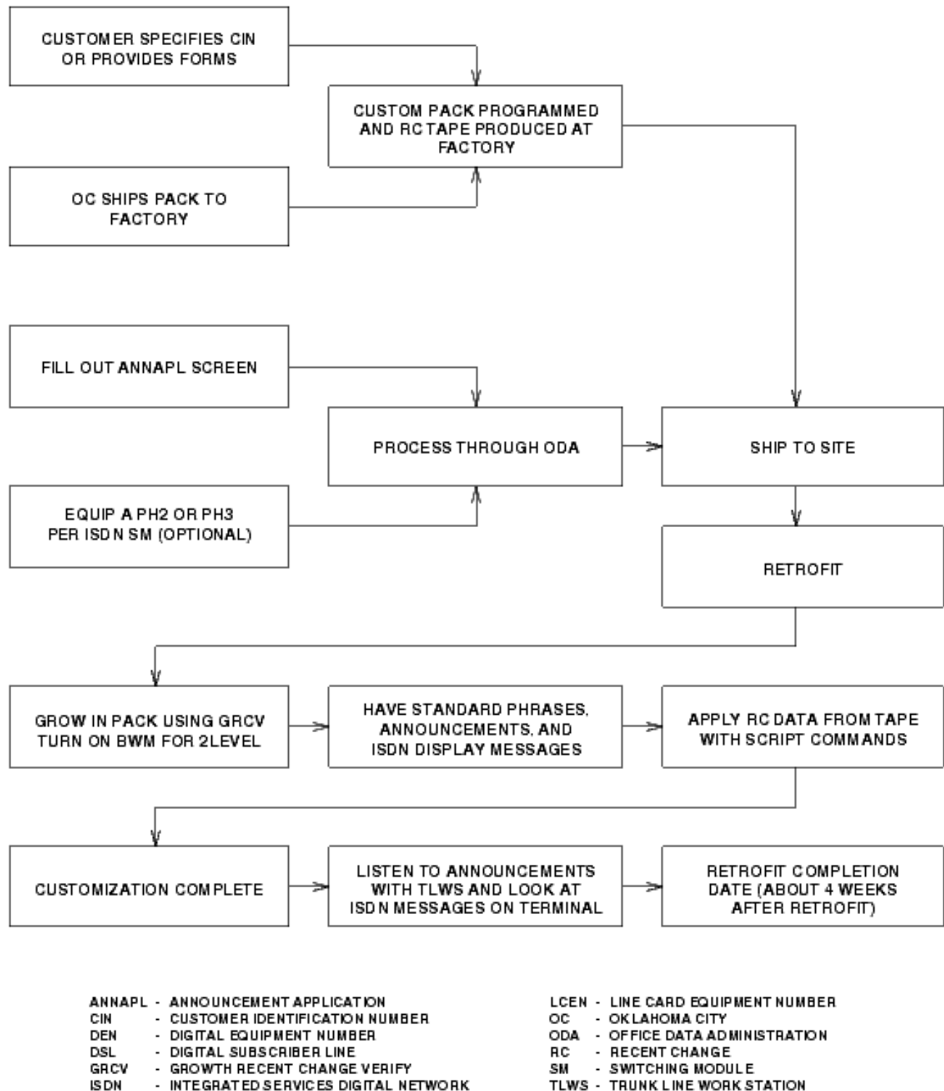
Figure 8-3 Custom Announcement (Retrofit to 5E6)
