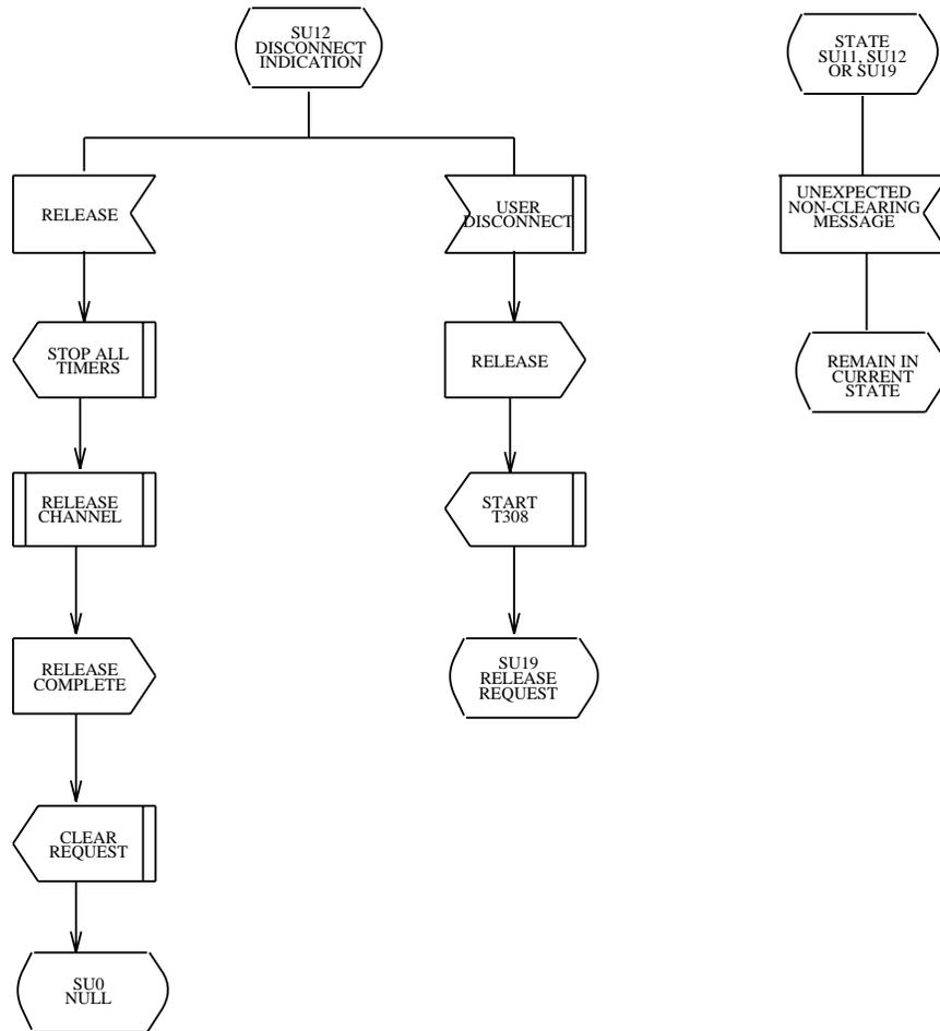
Figure 8-10 — Symmetrical User: SU12, Disconnect Indication State and Multiple States
