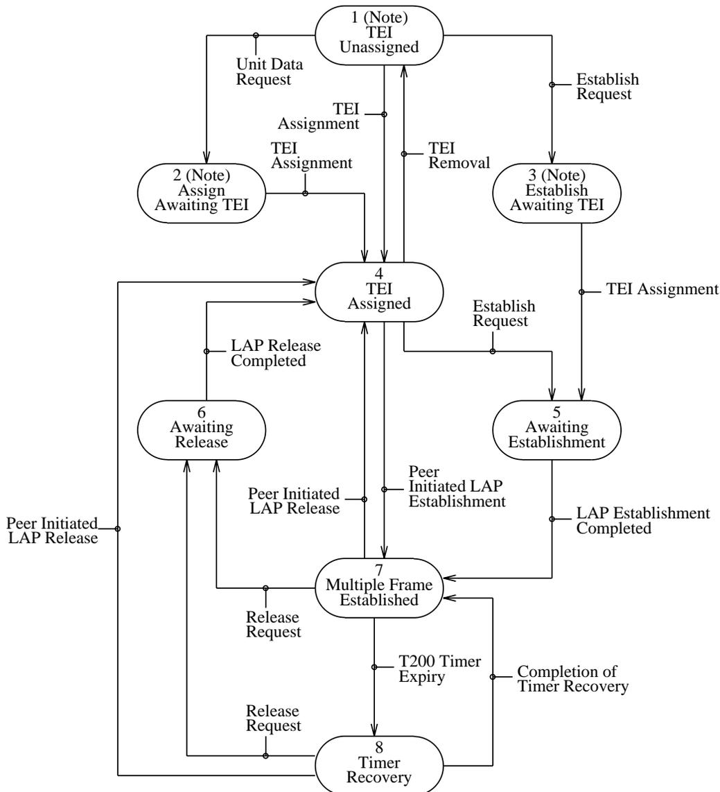
Note: States 1, 2, and 3 are not relevant to the primary interface because the TEI assignment procedures are not supported.
