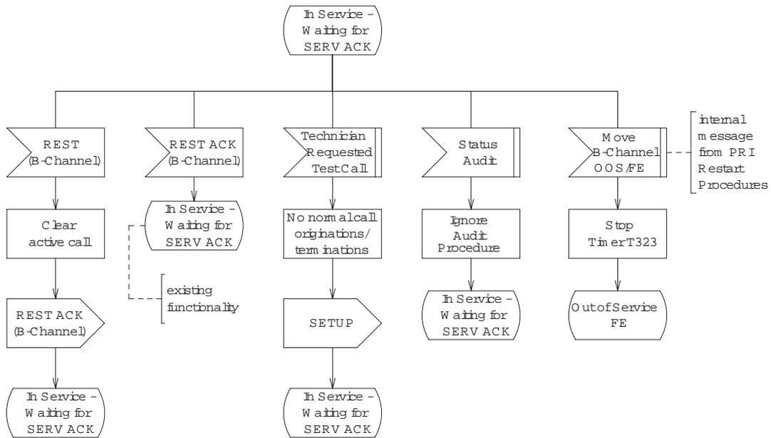
Figure 9.3-20 — National ISDN PRI with BCAS: B-channels, In Service, Waiting for SERV ACK (3 of 3)
