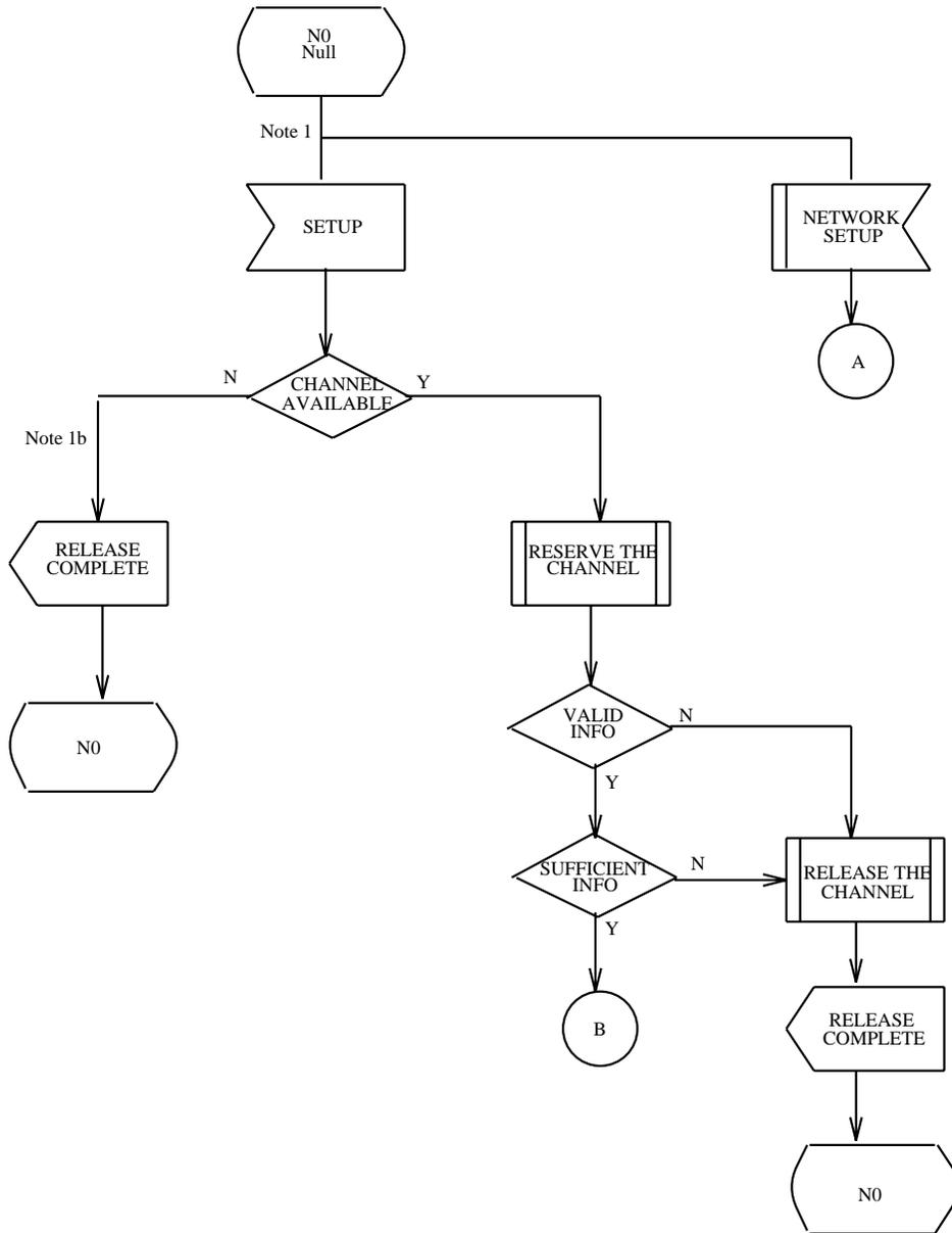
Figure 7-2 — Network Side: N0, Null State (1 of 2)
