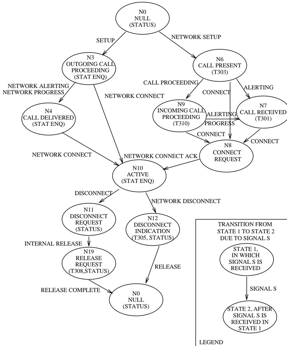
Figure 5.1-3 — Call States and Normal Transitions for Network Side
