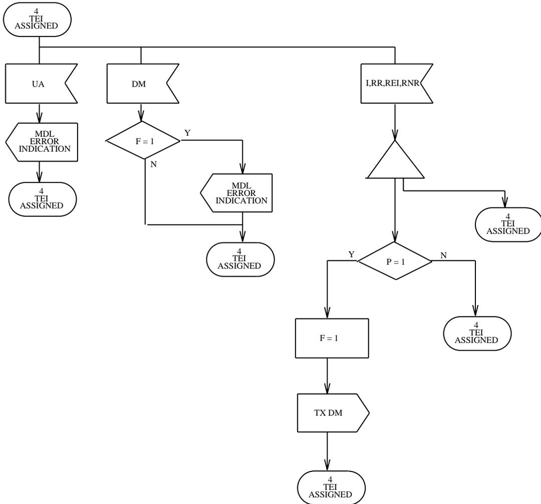
Figure 3.7-3 — Link Layer Point-to-Point: State 4, TEI Assigned (2 of 2)
