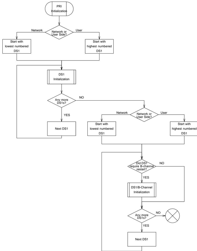
Figure 9.3-9 — National ISDN PRI with BCAS: Initialization Procedure
