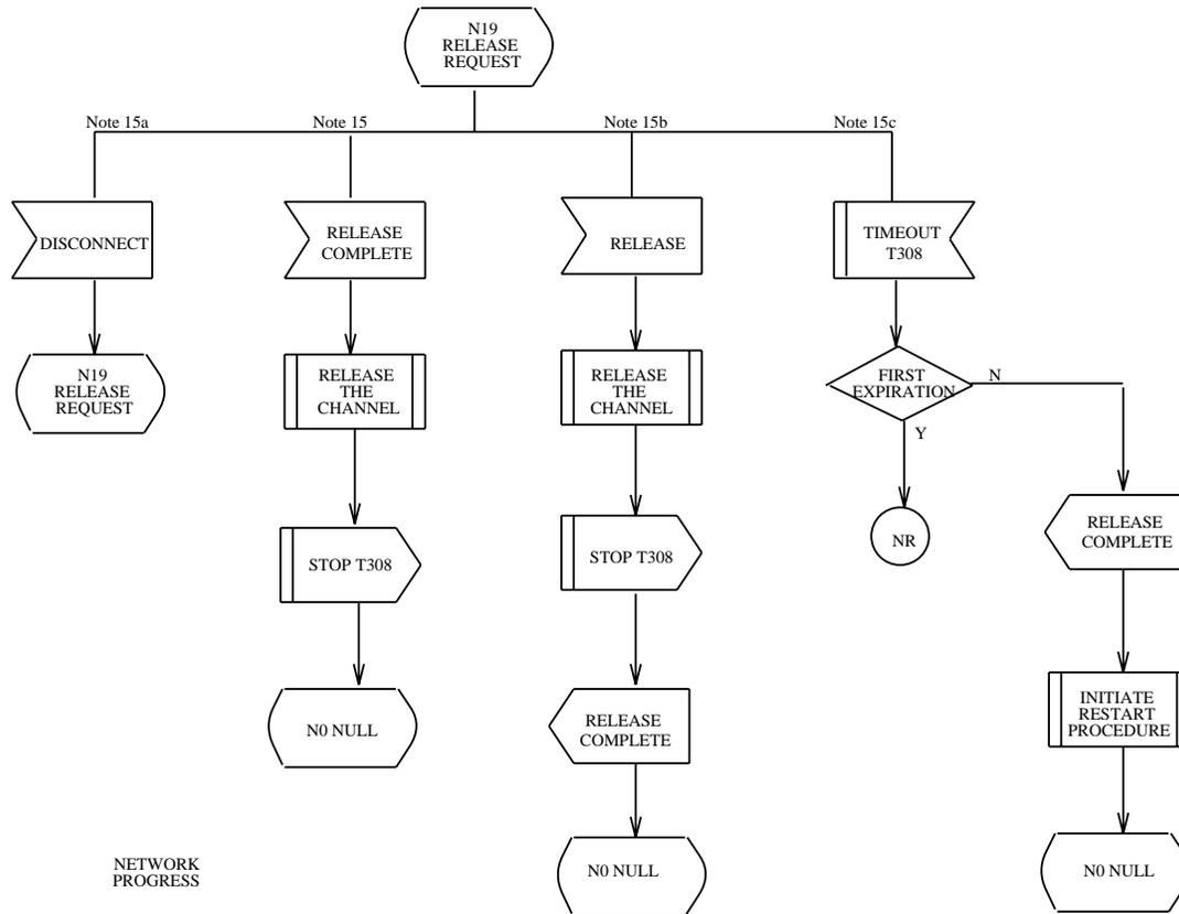
Figure 7-13 — Network Side: States N19, Release Request State
