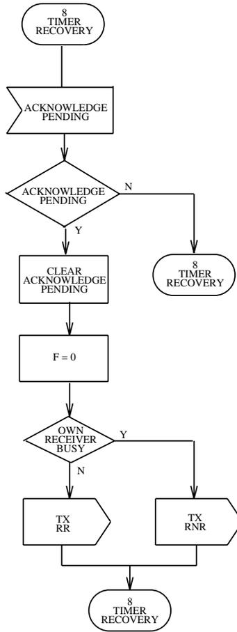
Figure 3.7-7 — Link Layer Point-to-Point: State 8, Timer Recovery (7 of 7)
