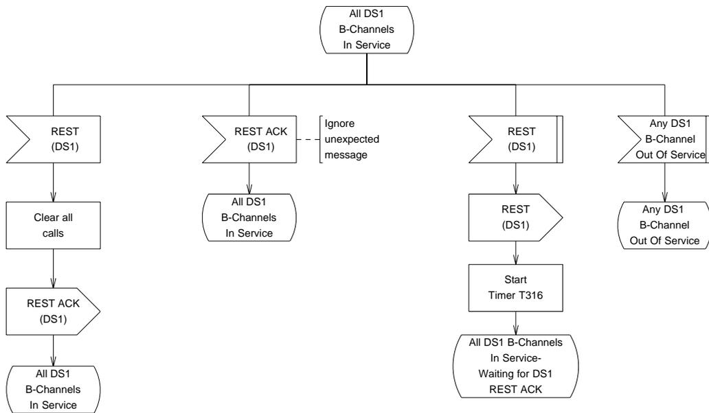
Figure 9.3-14 — National ISDN PRI with BCAS: DS1, All B-channels In Service State (1 of 2)
