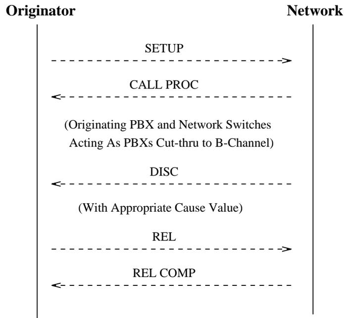
Figure 5.2-3 — Pure ISDN Network/PBX Call with Network Congestion
