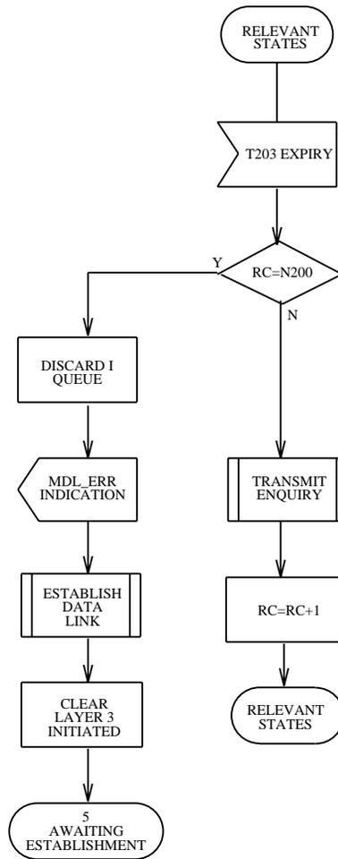
Figure 3.7-8 — Link Layer Point-to-Point: Relevant States (3 of 3)
