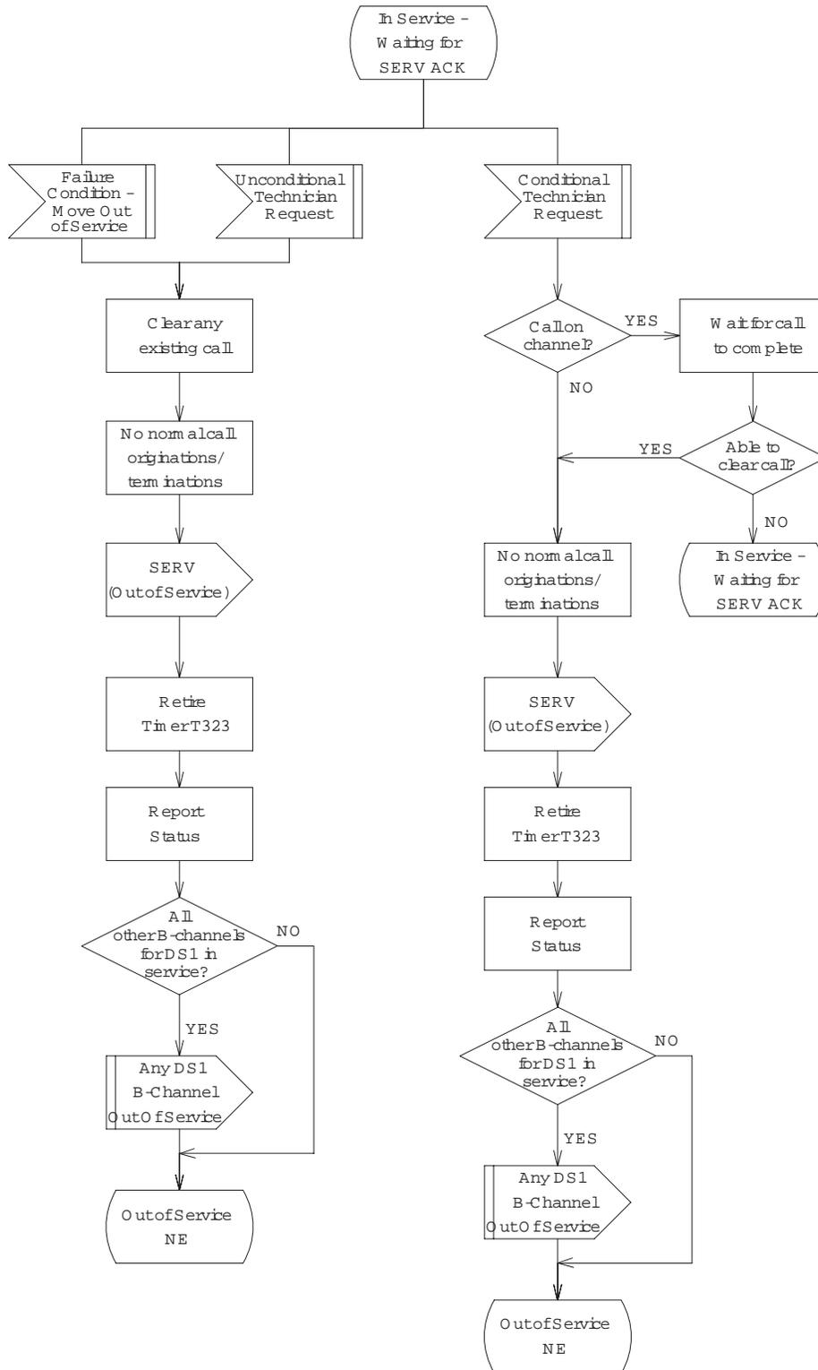
Figure 9.3-20 — National ISDN PRI with BCAS: B-channels, In Service, Waiting for SERV ACK (2 of 3)
