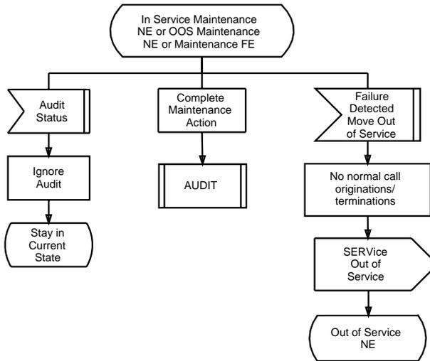
Figure 9.2-4 — Custom ISDN PRI: In Service Maintenance State (2 of 4)
