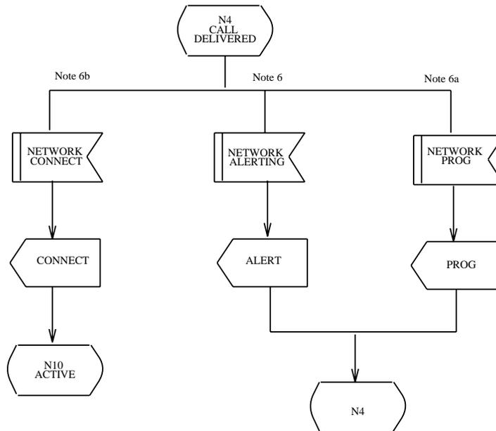
Figure 7-5 — Network Side: N4, Call Delivered State
