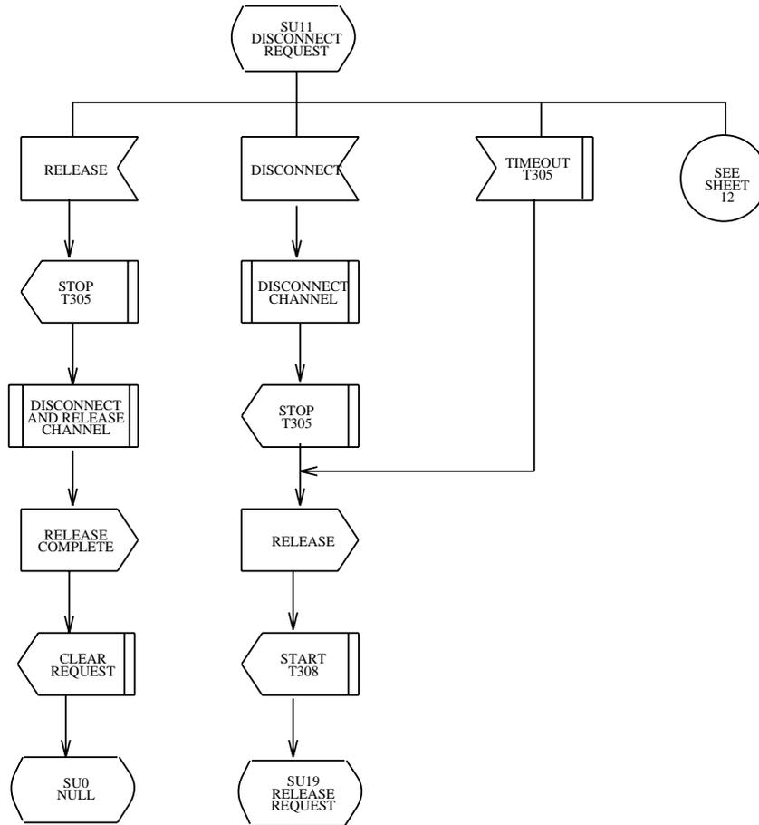
Figure 8-9 — Symmetrical User: SU11, Disconnect Request State
