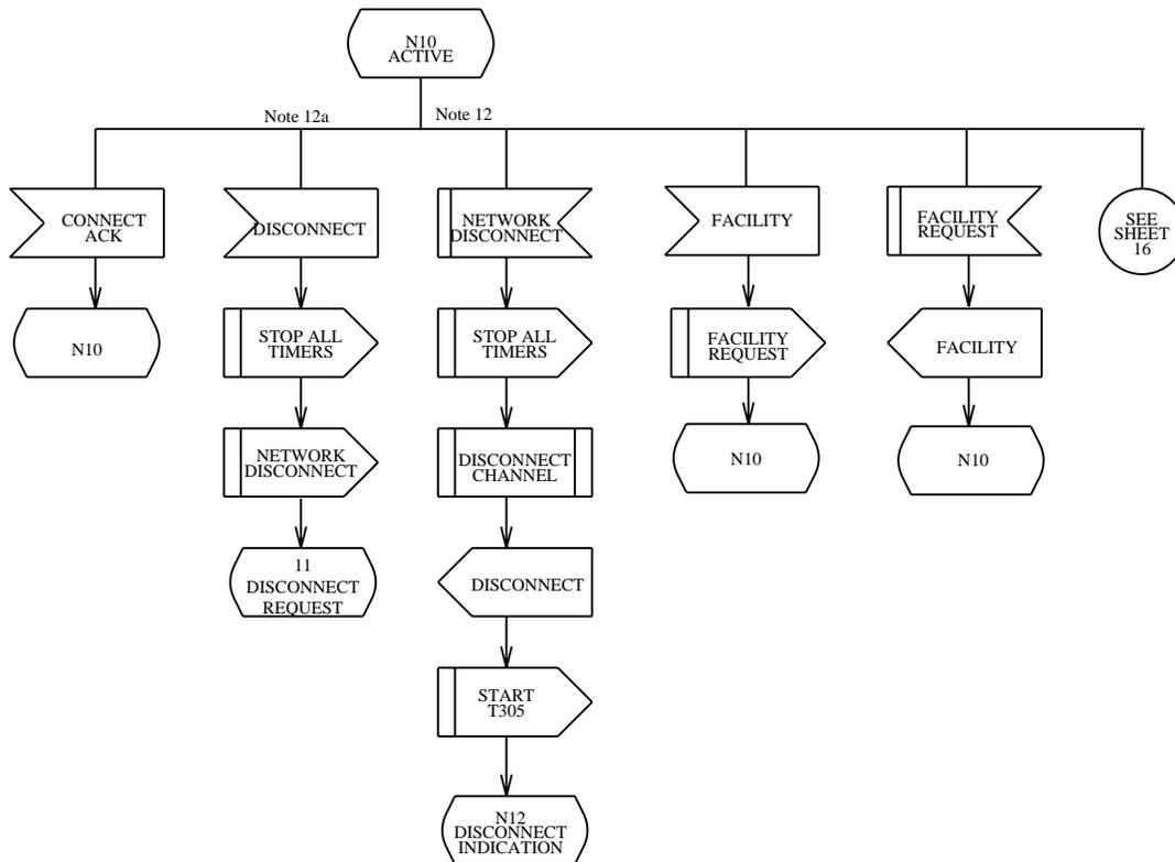
Figure 7-10 — Network Side: N10, Active State
