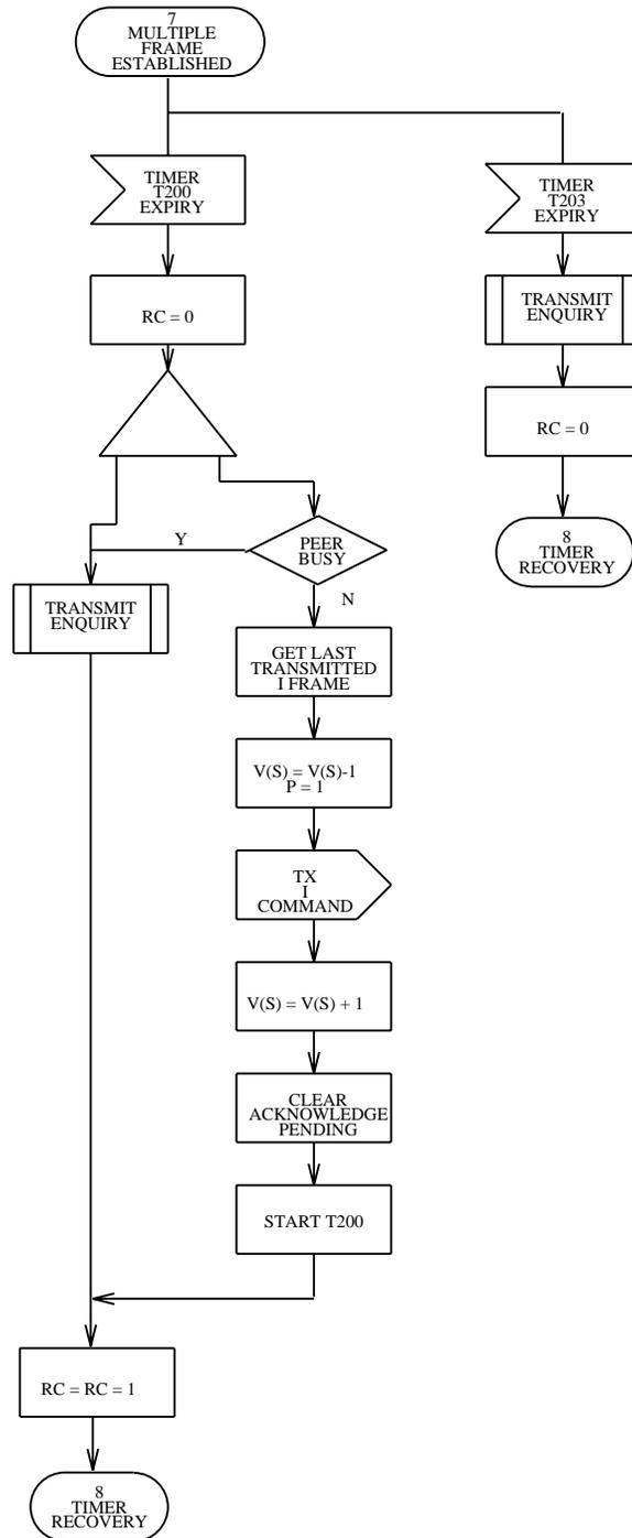
Figure 3.7-6 — Link Layer Point-to-Point: State 7, Multiple Frame Established (2 of 8)
