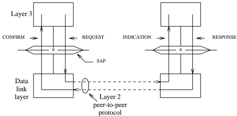
Figure 3.5-1 — Relationship of the Primitive Types to Layer 3 and the Data Link Layer
