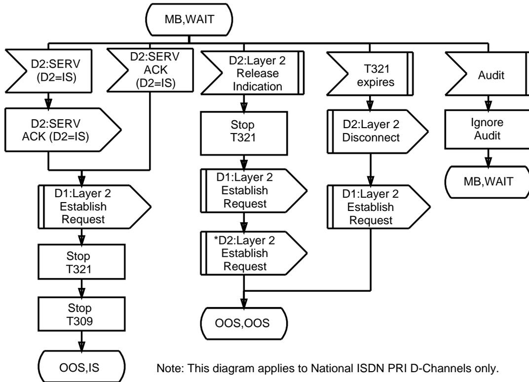
Figure 9.3-28 — National ISDN PRI with D-channel Backup: Maintenance Busy, WAIT (1 of 2)
