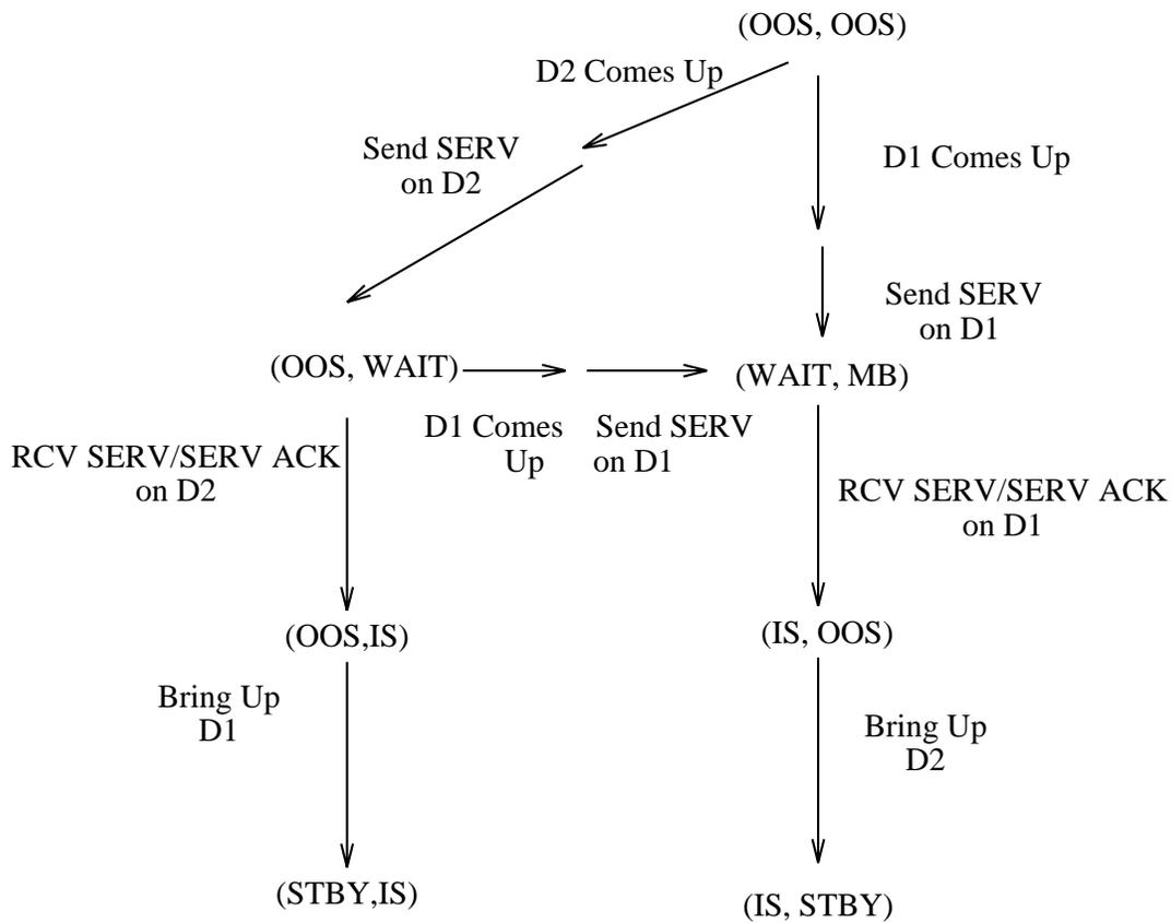
Figure 10-2 — Initialization Procedure
