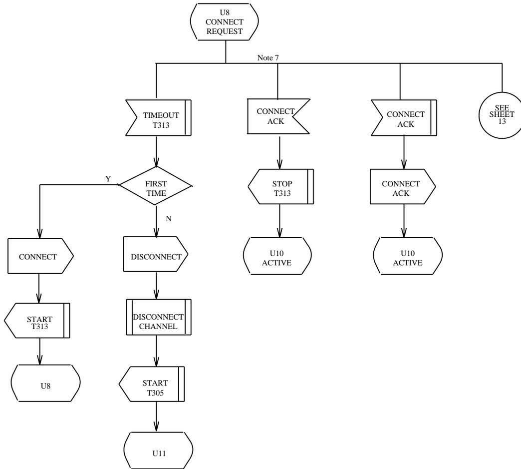
Figure 6-7 — User Side: U8, Connect Request State
