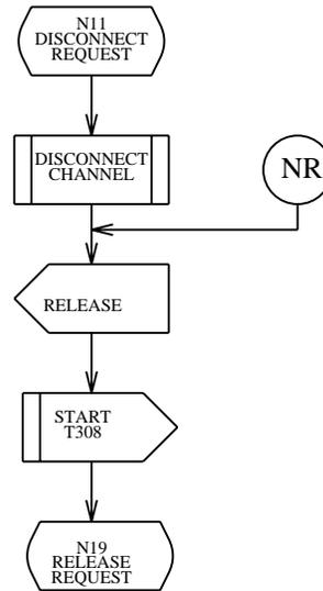
Figure 7-15 — Network Side: N11, Disconnect Request State
