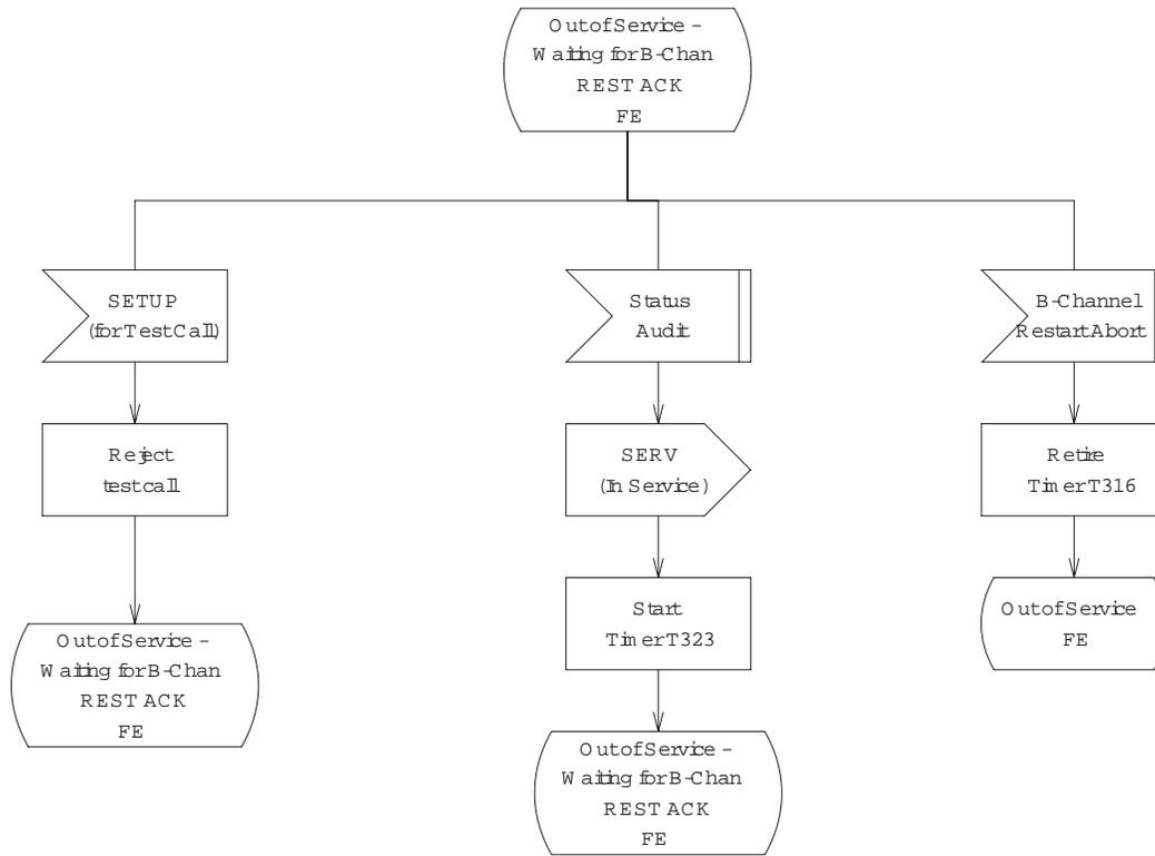
Figure 9.3-24 — National ISDN PRI with BCAS: B-channels, Out of Service FE, Waiting for B-channel REST ACK (4 of 4)
