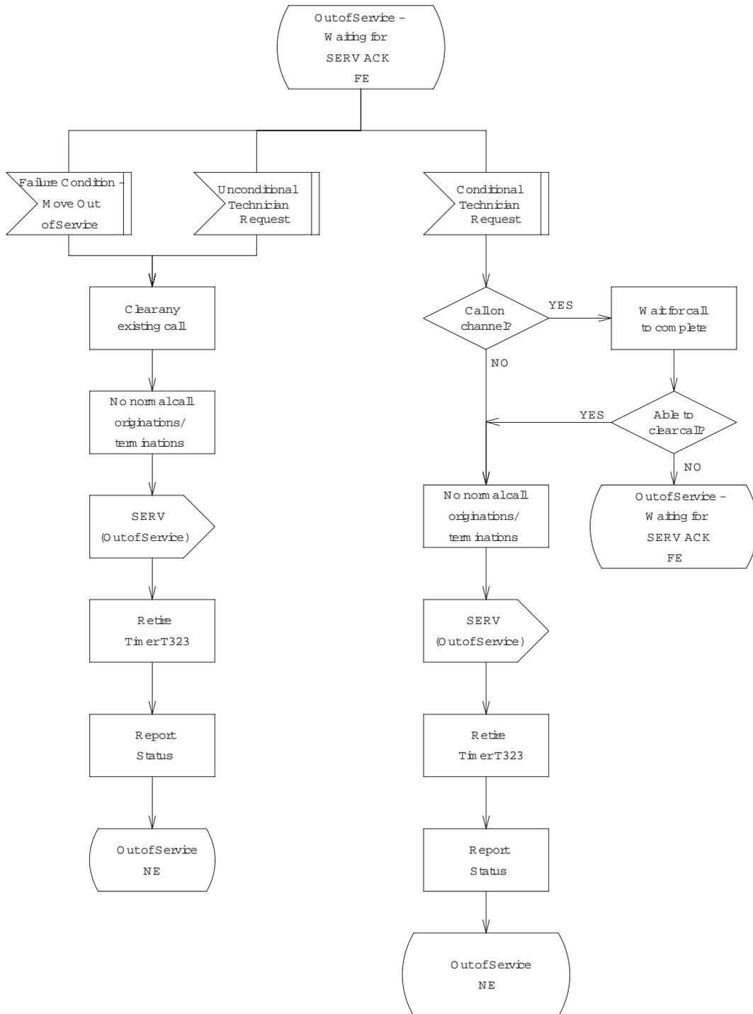
Figure 9.3-23 — National ISDN PRI with BCAS: B-channels, Out of Service FE, Waiting for SERV ACK (3 of 4)
