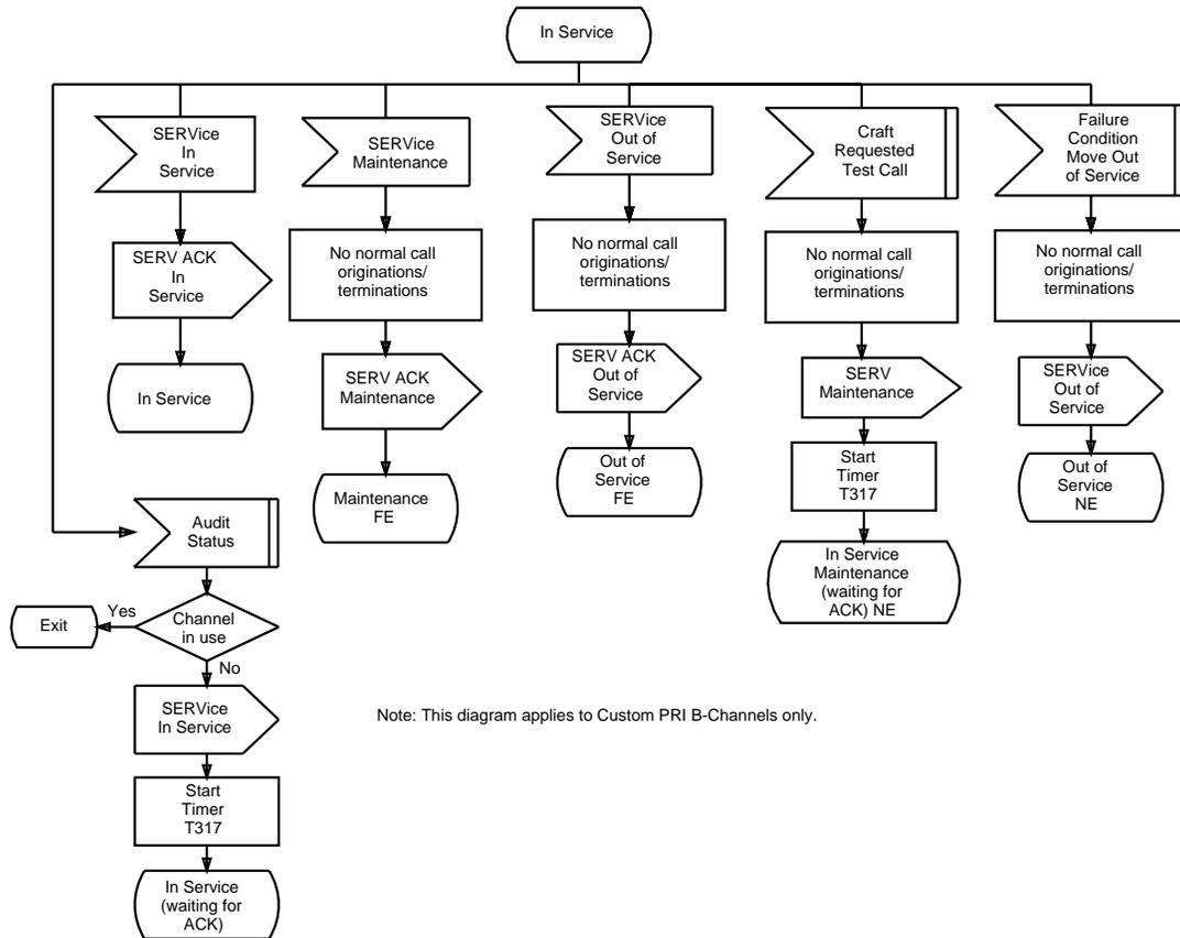
Figure 9.2-2 — Custom ISDN PRI: In Service State
