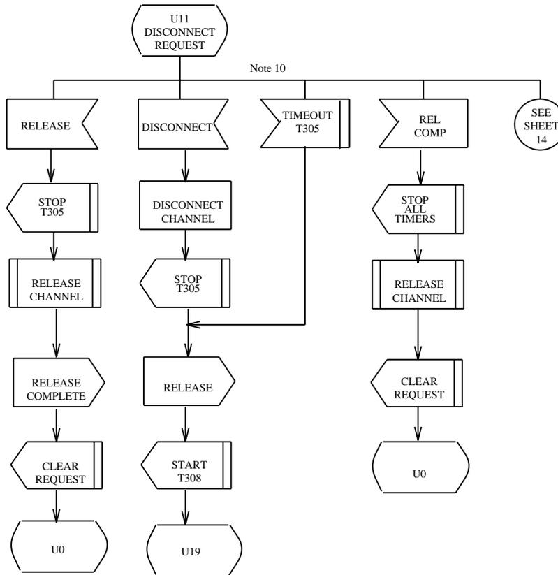
Figure 6-10 — User Side: U11, Disconnect Request State
