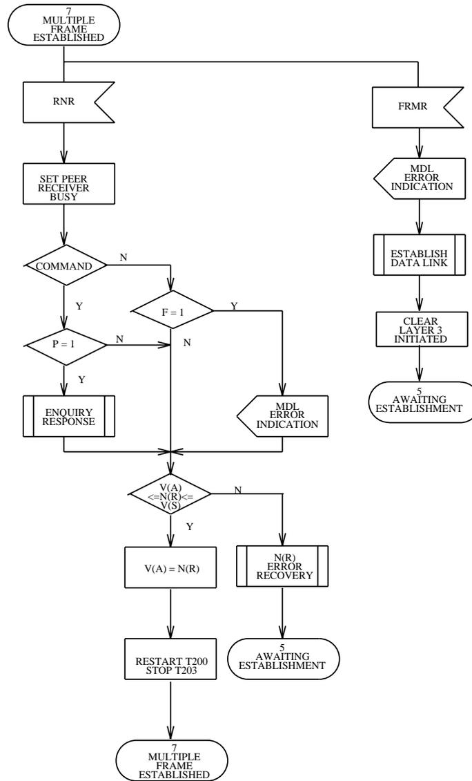
Figure 3.7-6 — Link Layer Point-to-Point: State 7, Multiple Frame Established (5 of 8)
