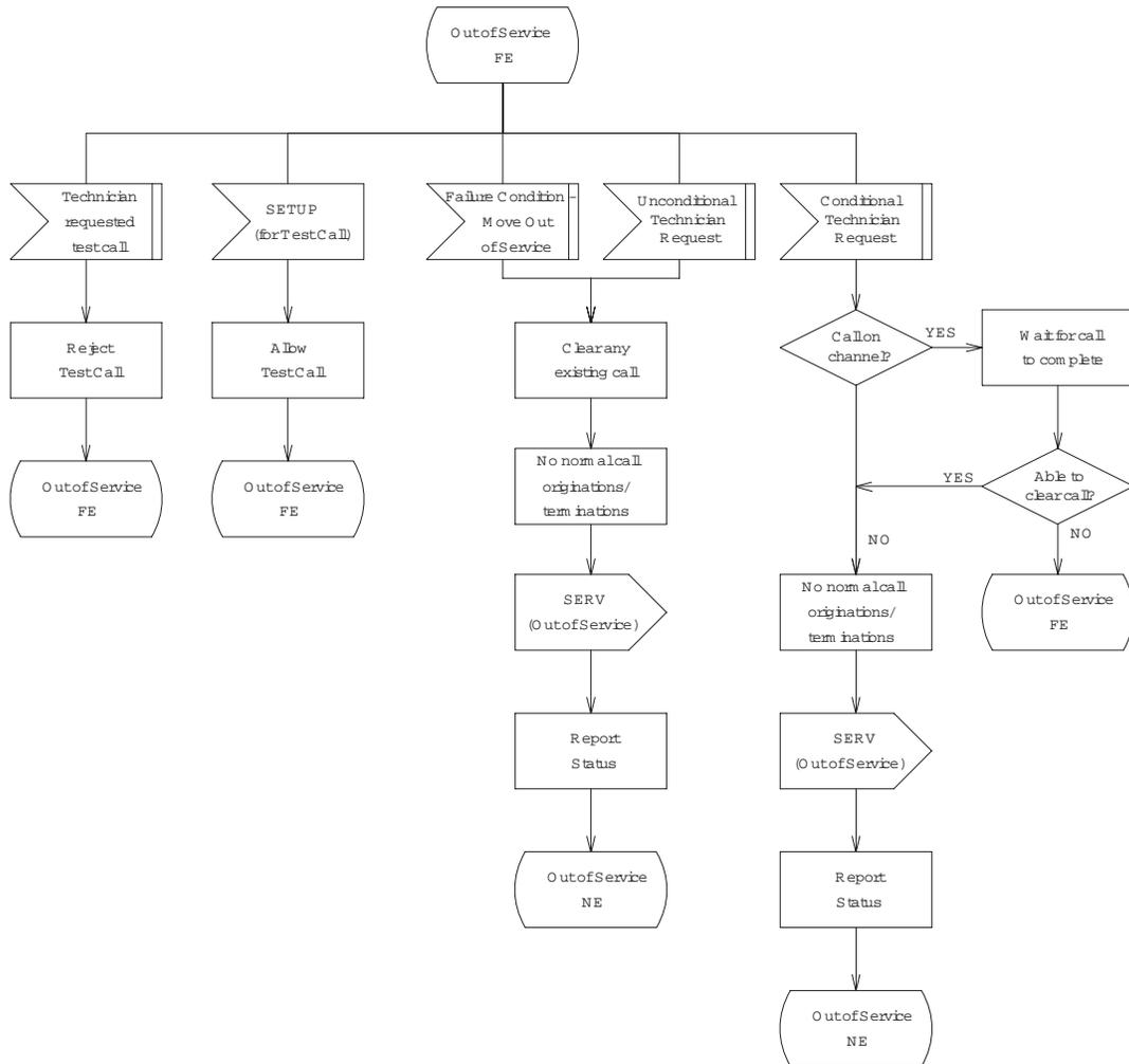
Figure 9.3-22 — National ISDN PRI with BCAS: B-channels, Out of Service FE (3 of 4)
