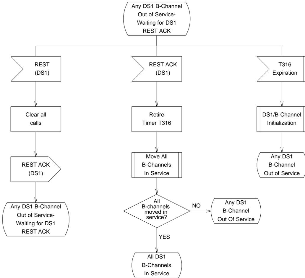
Figure 9.3-17 — National ISDN PRI with BCAS: DS1, Any B-channel Out of Service State, Waiting for DS1 REST ACK
