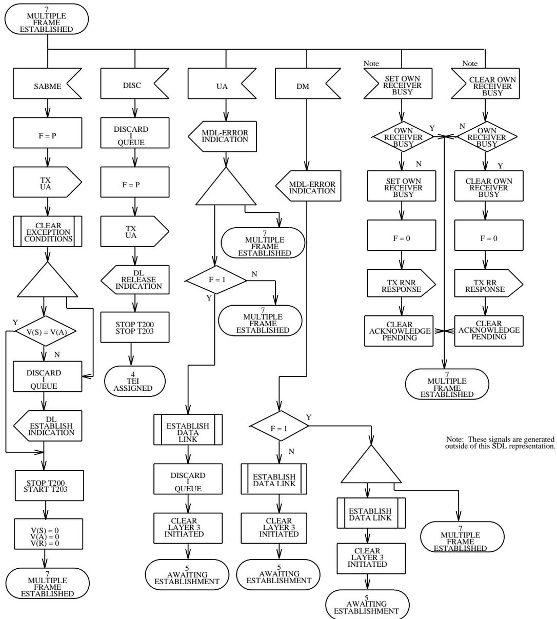
Figure 3.7-6 — Link Layer Point-to-Point: State 7, Multiple Frame Established (3 of 8)
