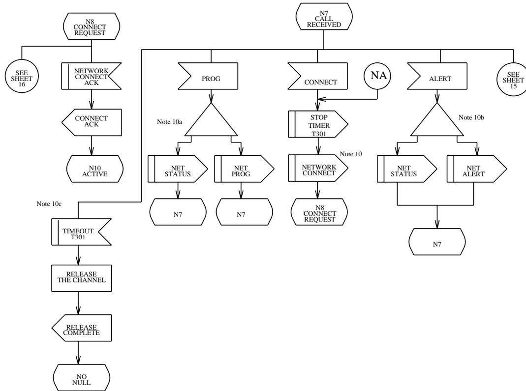
Figure 7-8 — Network Side: N7, Call Received State and N8, Connect Request State
