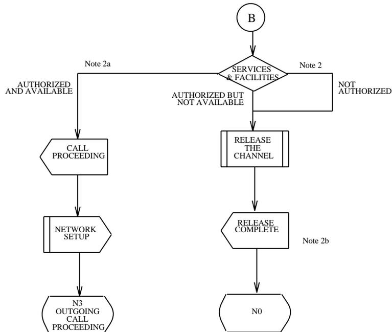
Figure 7-2 — Network Side: N0, Null State (2 of 2)
