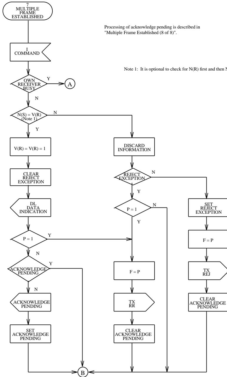
Figure 3.7-6 — Link Layer Point-to-Point: State 7, Multiple Frame Established (6 of 8)
