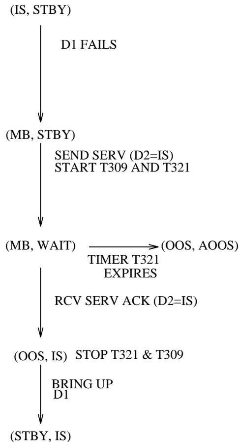
Figure 10-3 — Normal Switch-Over
