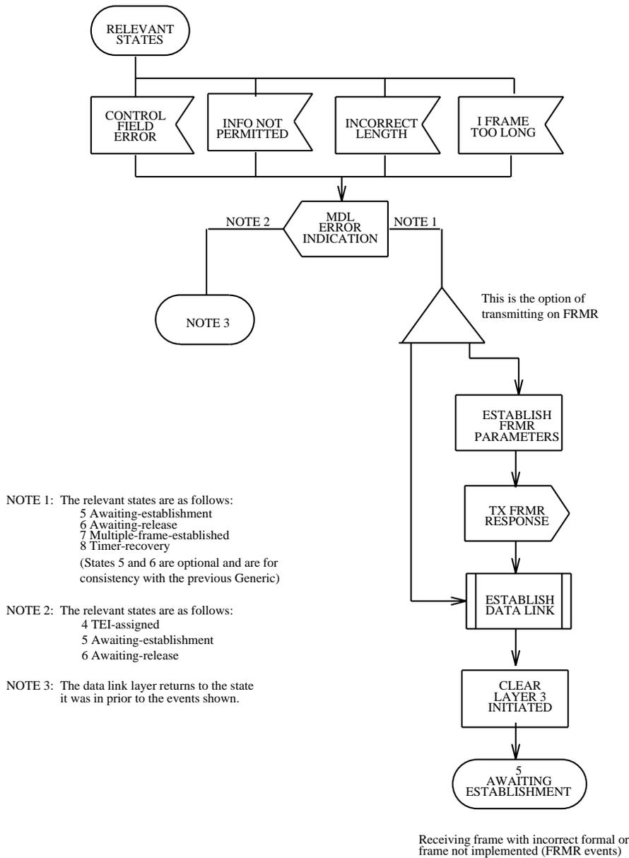
Figure 3.7-8 — Link Layer Point-to-Point: Relevant States (2 of 3)
