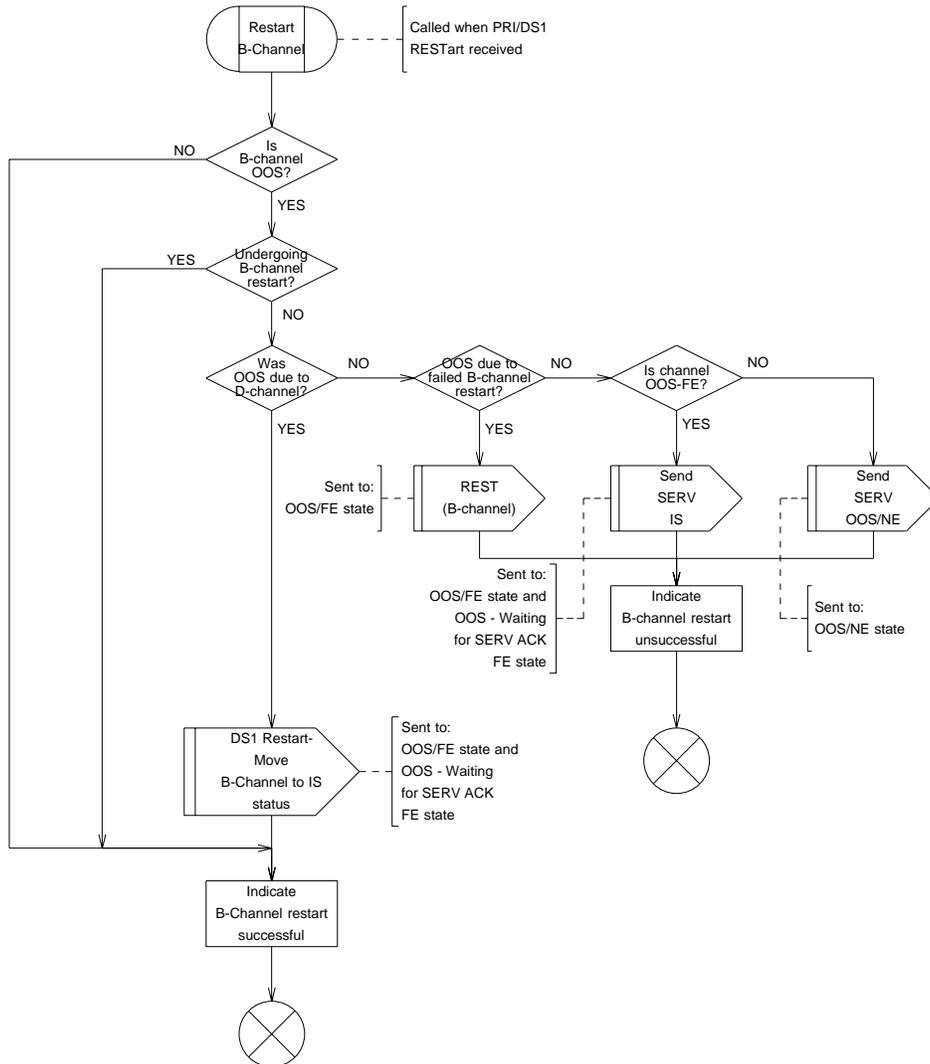
Figure 9.3-12 — National ISDN PRI with BCAS: Restart B-channel Procedure
