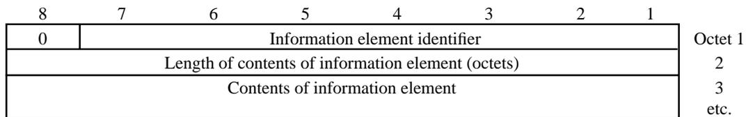
**Figure 4.3-2 — Variable Length Information Element Format**
