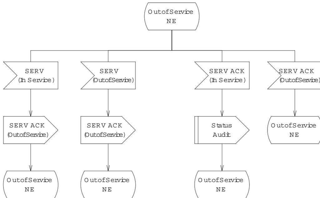
Figure 9.3-21 — National ISDN PRI with BCAS: B-channels, Out of Service NE (1 of 3)
