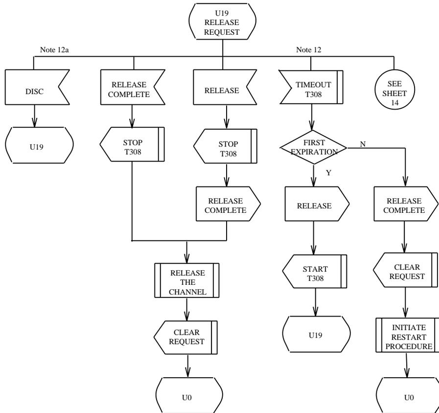
Figure 6-12 — User Side: U19, Release Request State
