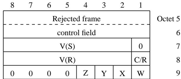
**Figure 3.4-2 — FRMR Information Field Format—Extended (Modulo 128) Operation**
