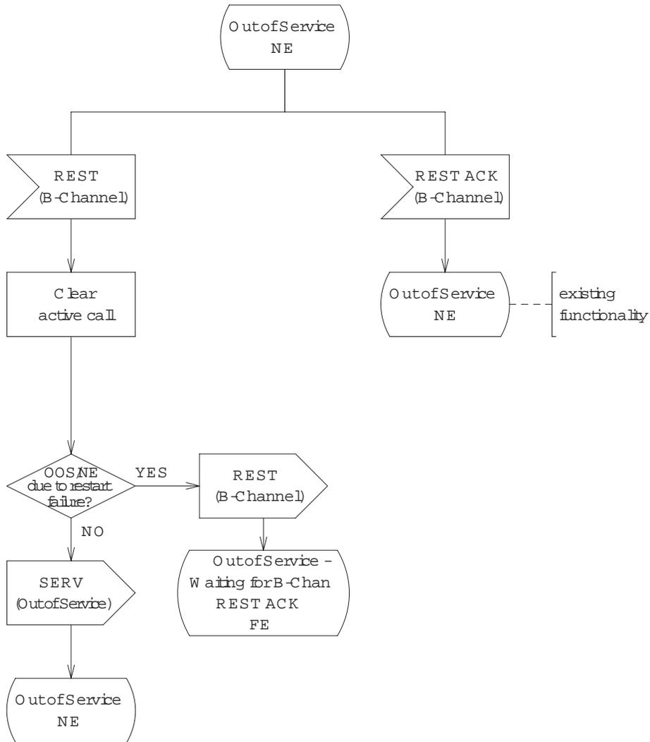
Figure 9.3-21 — National ISDN PRI with BCAS: B-channels, Out of Service NE (2 of 3)
