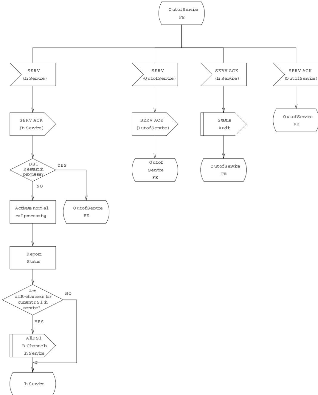
Figure 9.3-22 — National ISDN PRI with BCAS: B-channels, Out of Service FE (1 of 4)
