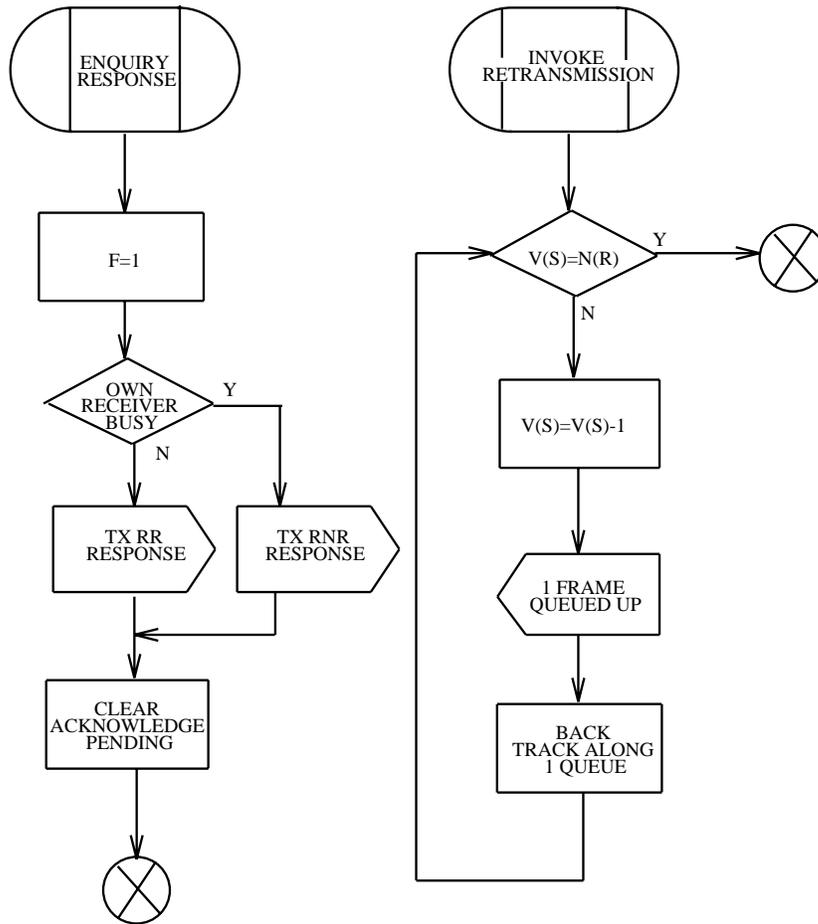
NOTE: The generation of the correct number of signals in order to cause the required retransmission of I frames does not alter their sequence integrity.
