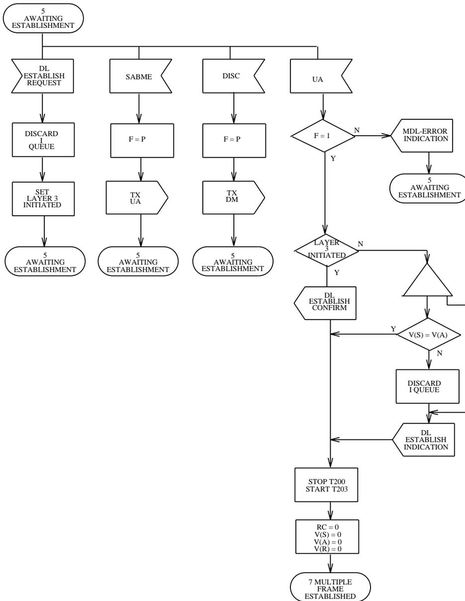
Figure 3.7-4 — Link Layer Point-to-Point: State 5, Awaiting Establishment (1 of 2)
