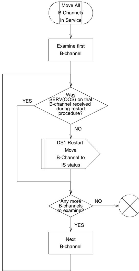
Figure 9.3-18 — National ISDN PRI with BCAS: DS1, Move All B-channels In Service
