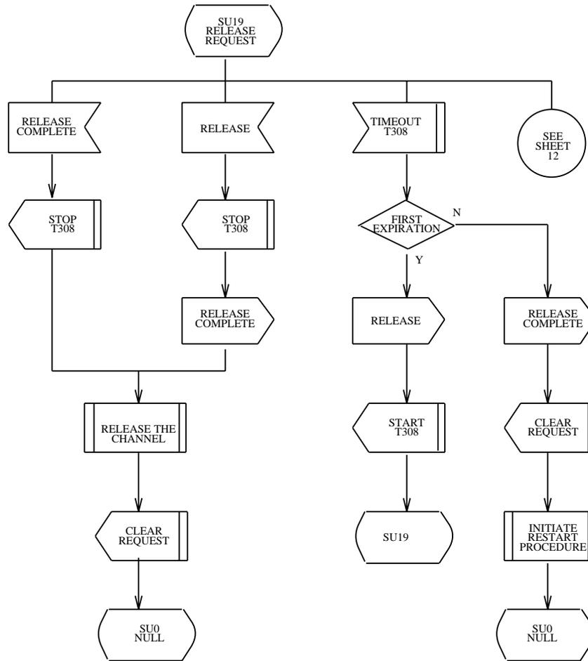
Figure 8-11 — Symmetrical User: SU19, Release Request State
