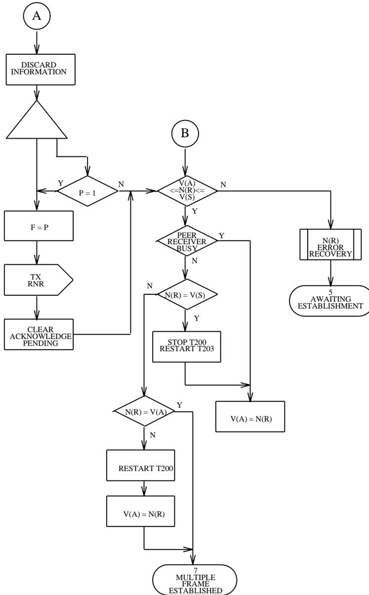
Figure 3.7-6 — Link Layer Point-to-Point: State 7, Multiple Frame Established (7 of 8)
