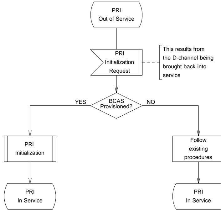
Figure 9.3-8 — National ISDN PRI with BCAS: Out of Service State
