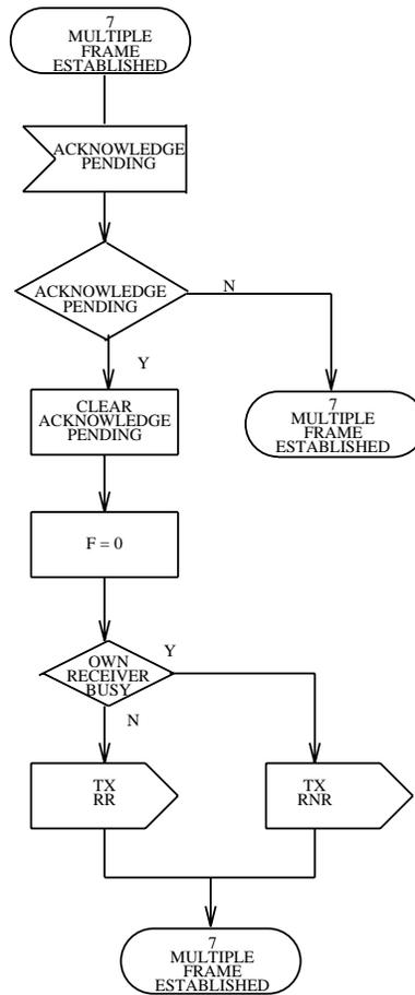
Figure 3.7-6 — Link Layer Point-to-Point: State 7, Multiple Frame Established (8 of 8)
