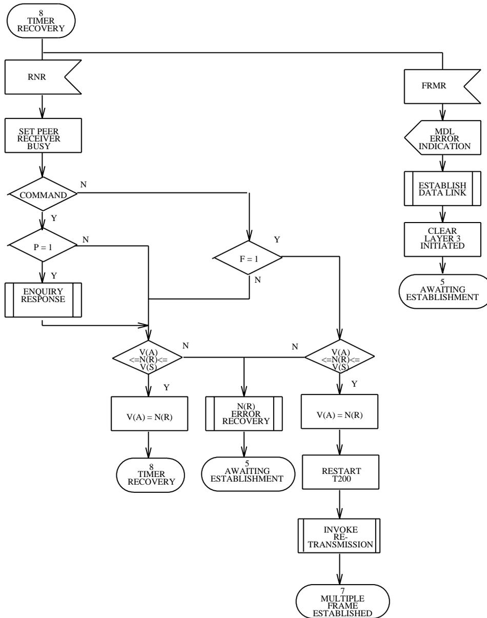
Figure 3.7-7 — Link Layer Point-to-Point: State 8, Timer Recovery (4 of 7)
