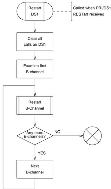
Figure 9.3-11 — National ISDN PRI with BCAS: Restart DS1 Procedure
