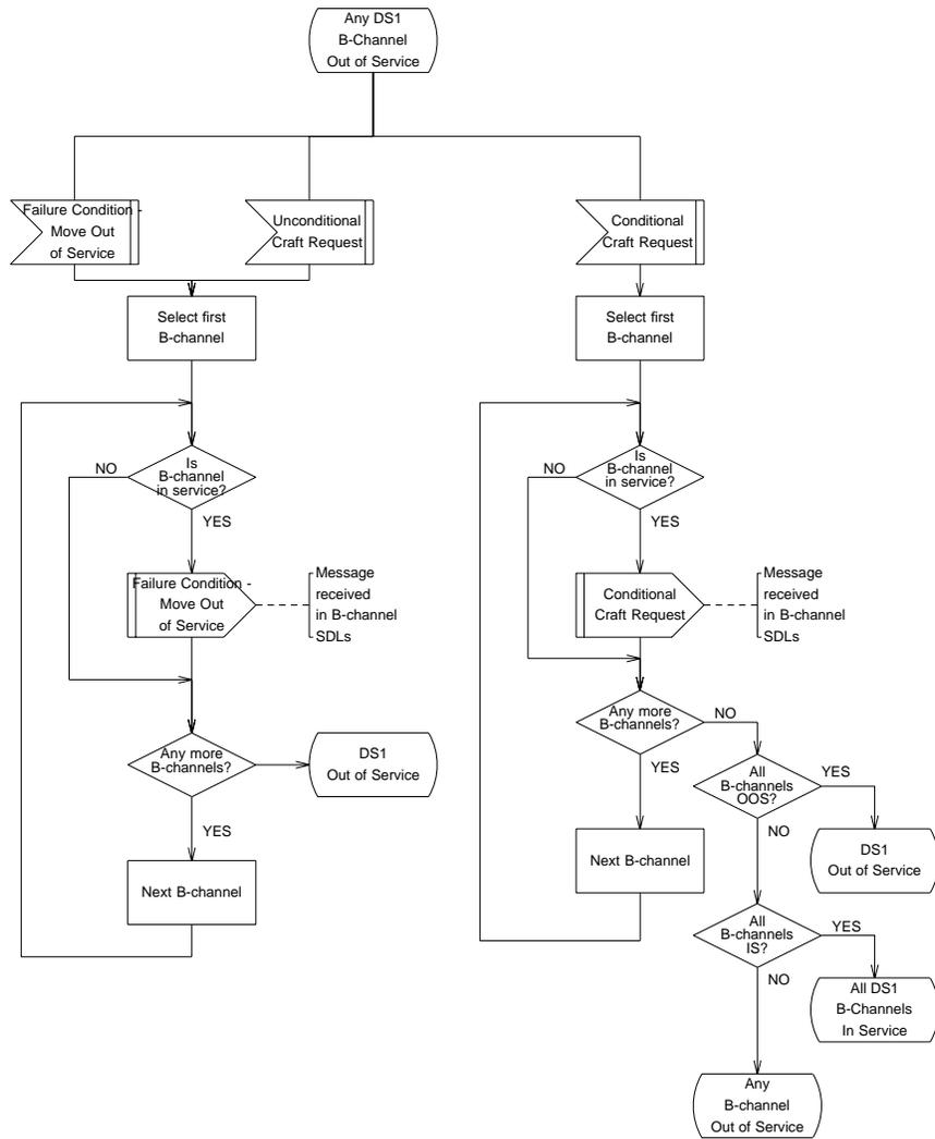
Figure 9.3-16 — National ISDN PRI with BCAS: DS1, Any B-channel Out of Service State (2 of 2)
