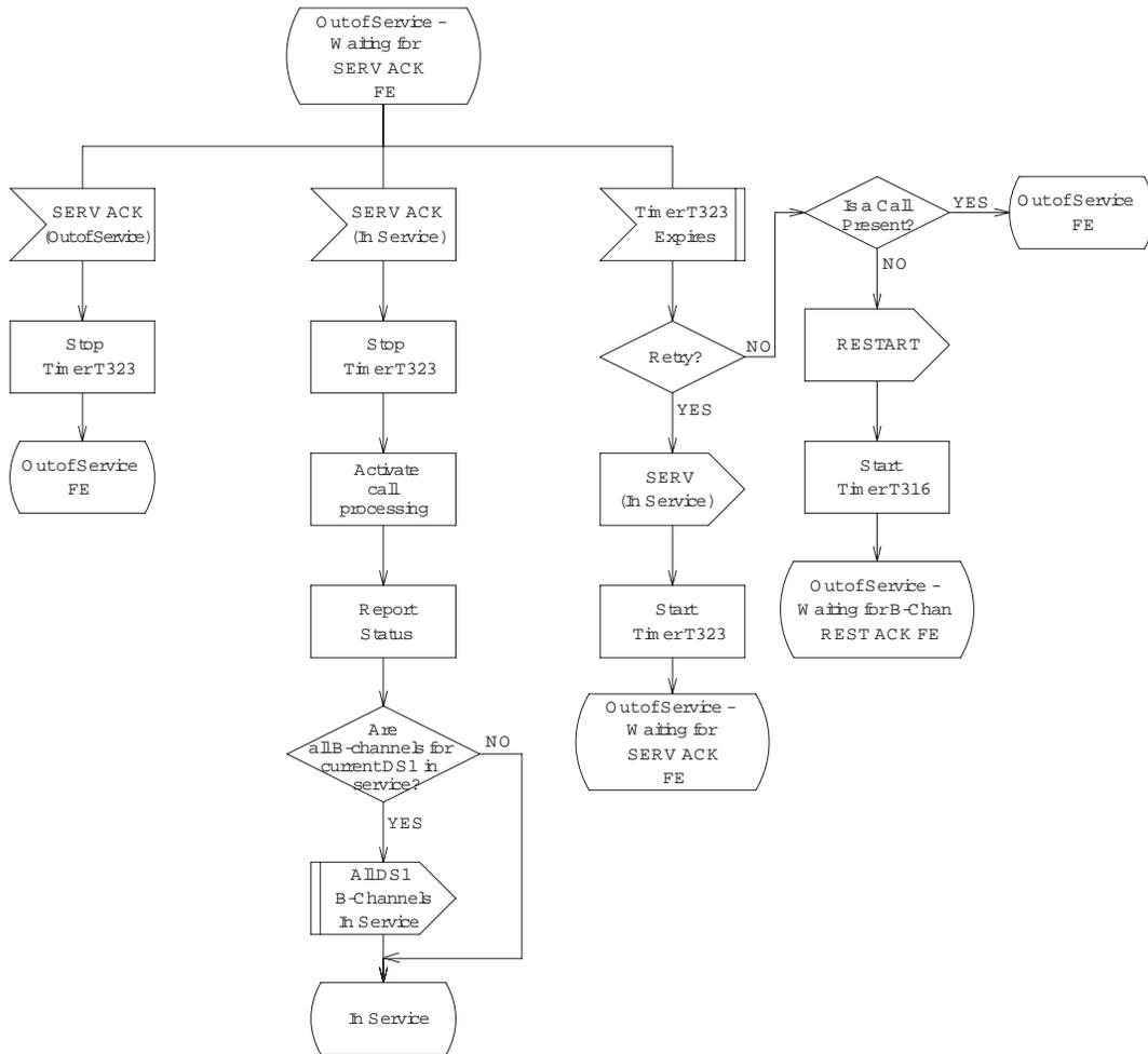
Figure 9.3-23 — National ISDN PRI with BCAS: B-channels, Out of Service FE, Waiting for SERV ACK (1 of 4)
