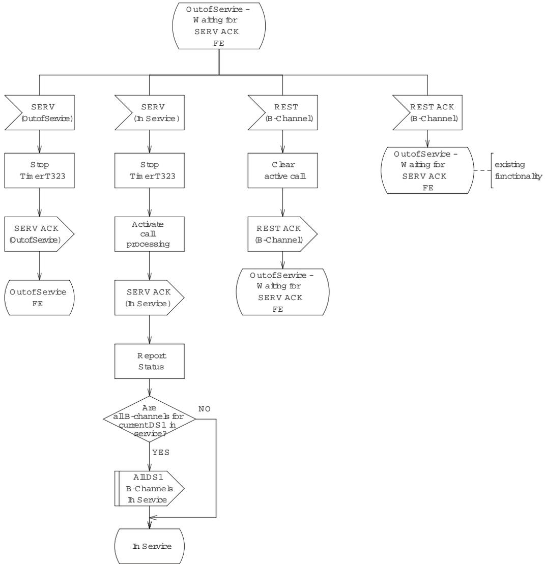
Figure 9.3-23 — National ISDN PRI with BCAS: B-channels, Out of Service FE, Waiting for SERV ACK (2 of 4)
