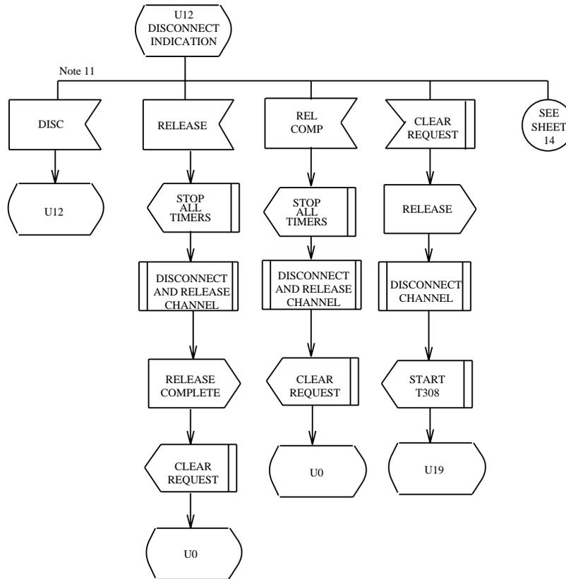
Figure 6-11 — User Side: U12, Disconnect Indication State
