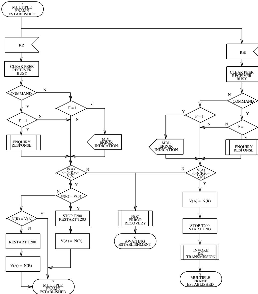
Figure 3.7-6 — Link Layer Point-to-Point: State 7, Multiple Frame Established (4 of 8)
