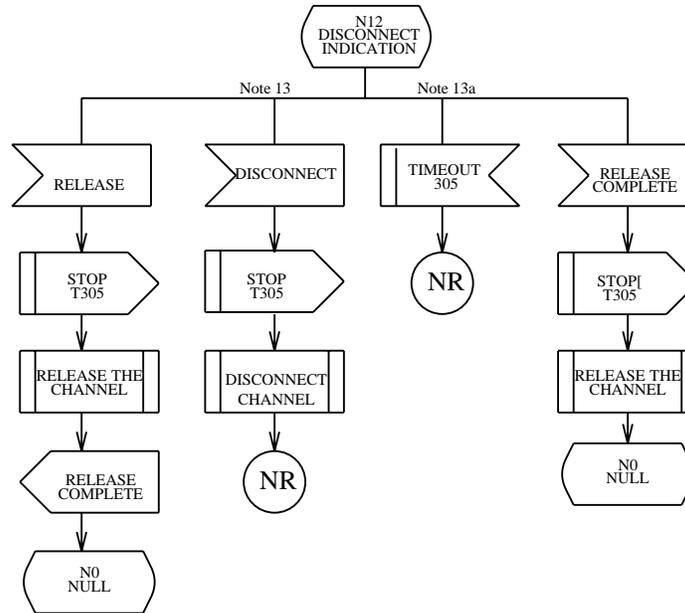
**Figure 7-11 — Network Side: N12, Disconnect Indication State**
