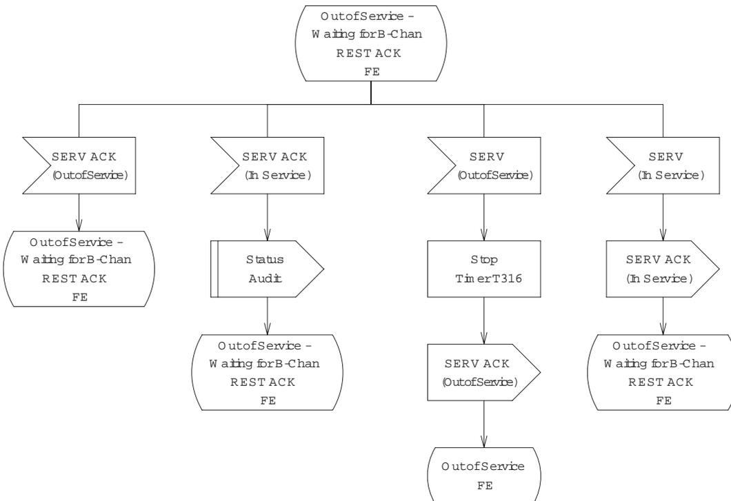
Figure 9.3-24 — National ISDN PRI with BCAS: B-channels, Out of Service FE, Waiting for B-channel REST ACK (1 of 4)
