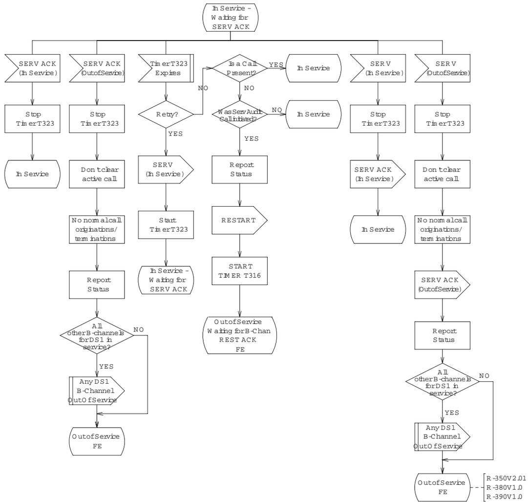
Figure 9.3-20 — National ISDN PRI with BCAS: B-channels, In Service, Waiting for SERV ACK (1 of 3)
