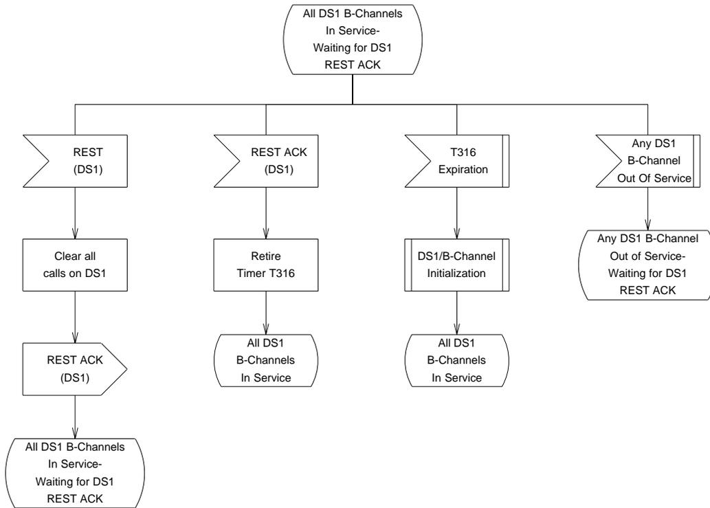
Figure 9.3-15 — National ISDN PRI with BCAS: DS1, All B-channels In Service State, Waiting for DS1 REST ACK
