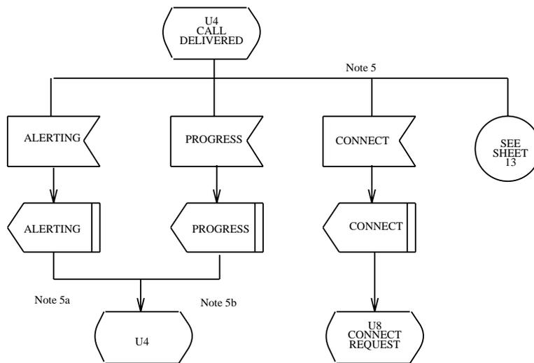
Figure 6-5 — User Side: U4, Call Delivered State
