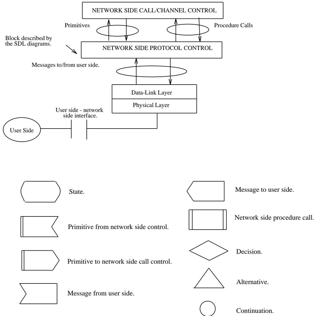
Figure 7-1 — Legend for Network Side Protocol Control SDL Diagrams
