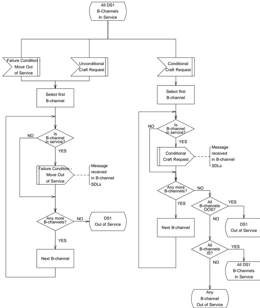
Figure 9.3-14 — National ISDN PRI with BCAS: DS1, All B-channels In Service State (2 of 2)
