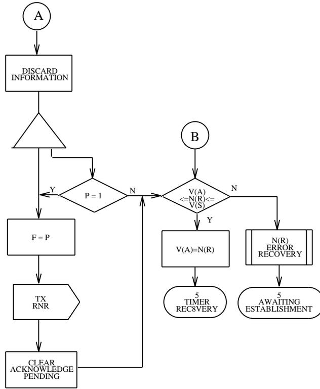
Figure 3.7-7 — Link Layer Point-to-Point: State 8, Timer Recovery (6 of 7)
