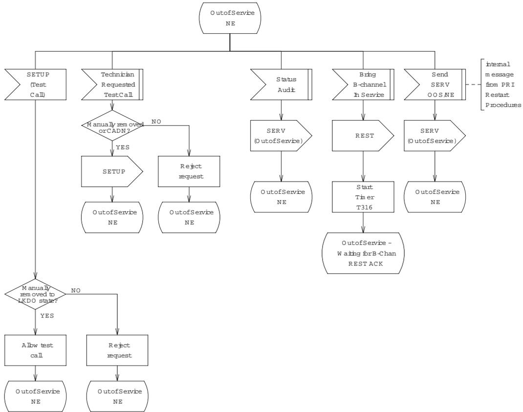
Figure 9.3-21 — National ISDN PRI with BCAS: B-channels, Out of Service NE (3 of 3)
