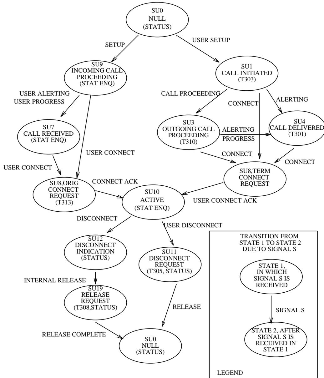
Figure 5.1-4 — Call States and Normal Transitions for Symmetrical User Side
