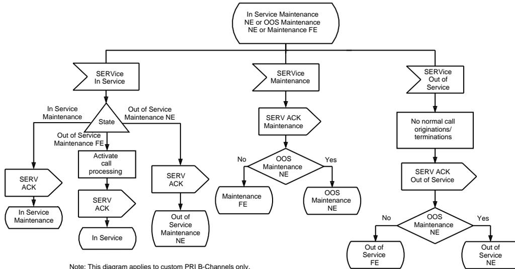
Figure 9.2-4 — Custom ISDN PRI: In Service Maintenance State (1 of 4)
