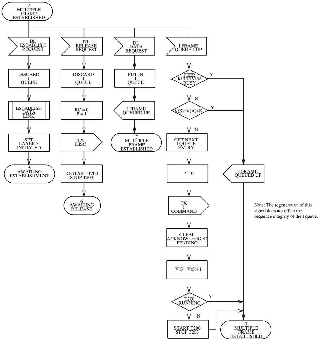
Figure 3.7-6 — Link Layer Point-to-Point: State 7, Multiple Frame Established (1 of 8)
