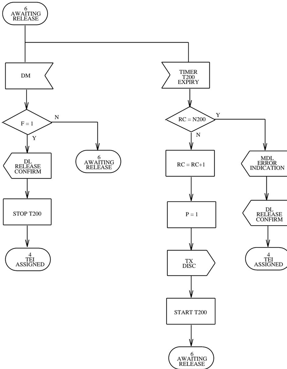
Figure 3.7-5 — Link Layer Point-to-Point: State 6, Awaiting Release (2 of 2)
