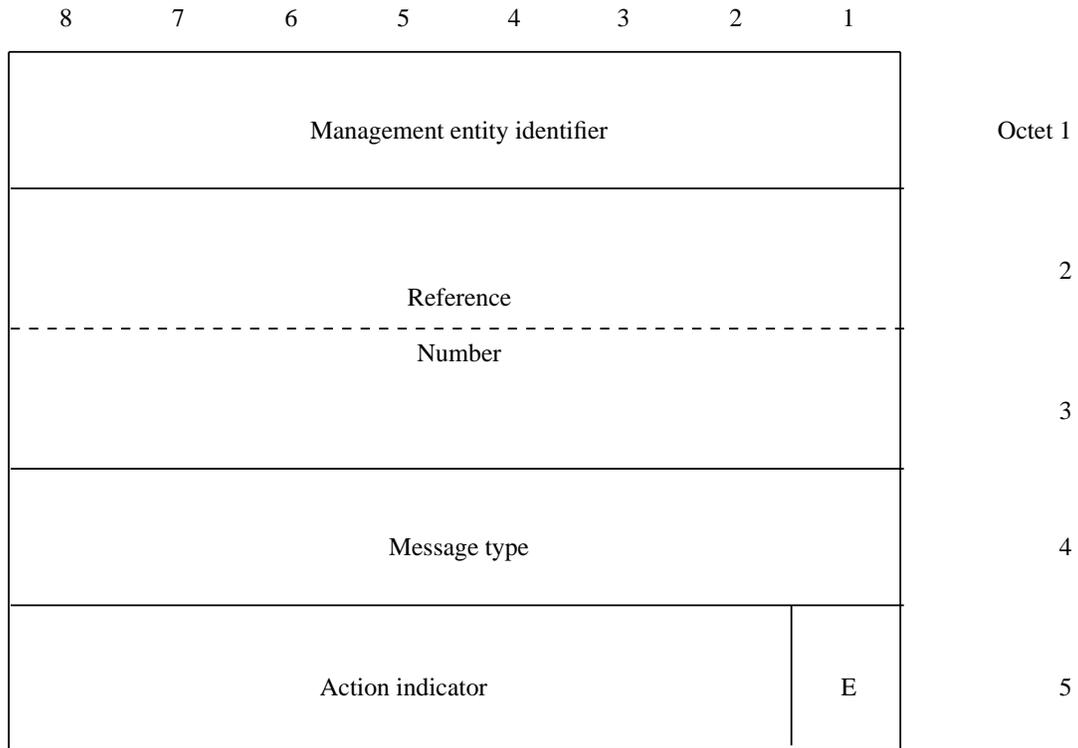
**Figure 3.6-1 — Message Structure for TEI Management Procedures**
