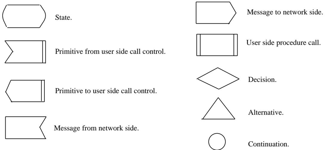
Figure 6-1 — Legend for User Side Protocol Control SDL Diagrams
