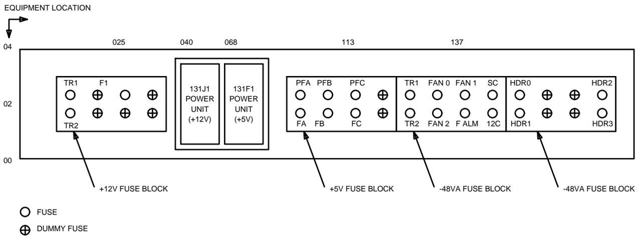
Figure 23. DSD8 Fuse Panel Unit J4A017HD-1 List 2
