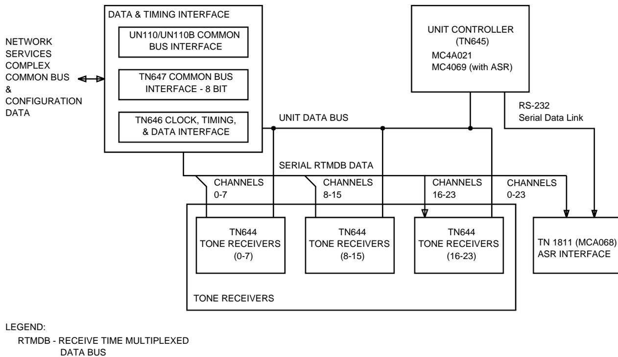
**Figure 35. Tone Receiver Unit — Functional Block Diagram (SD-4A116-01)**
