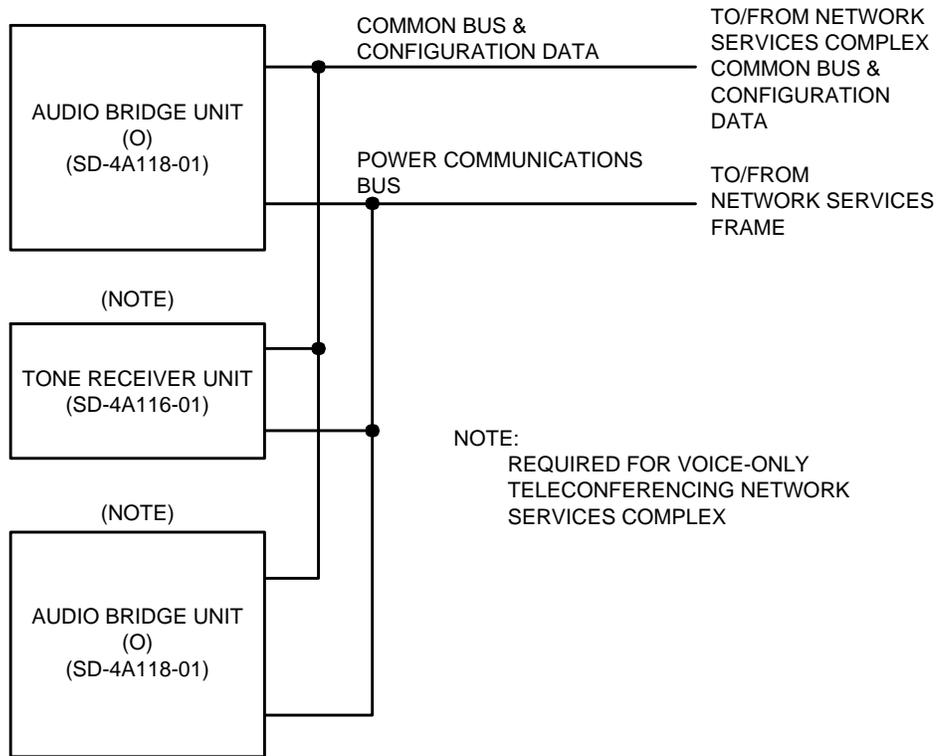
**Figure 36. Audio Bridge Frame — Functional Block Diagram (SD-4A117-01)**
