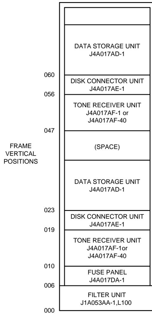
**Figure 14. Direct Services Dialing Frame J4A017H-1 — Equipment Identification**
