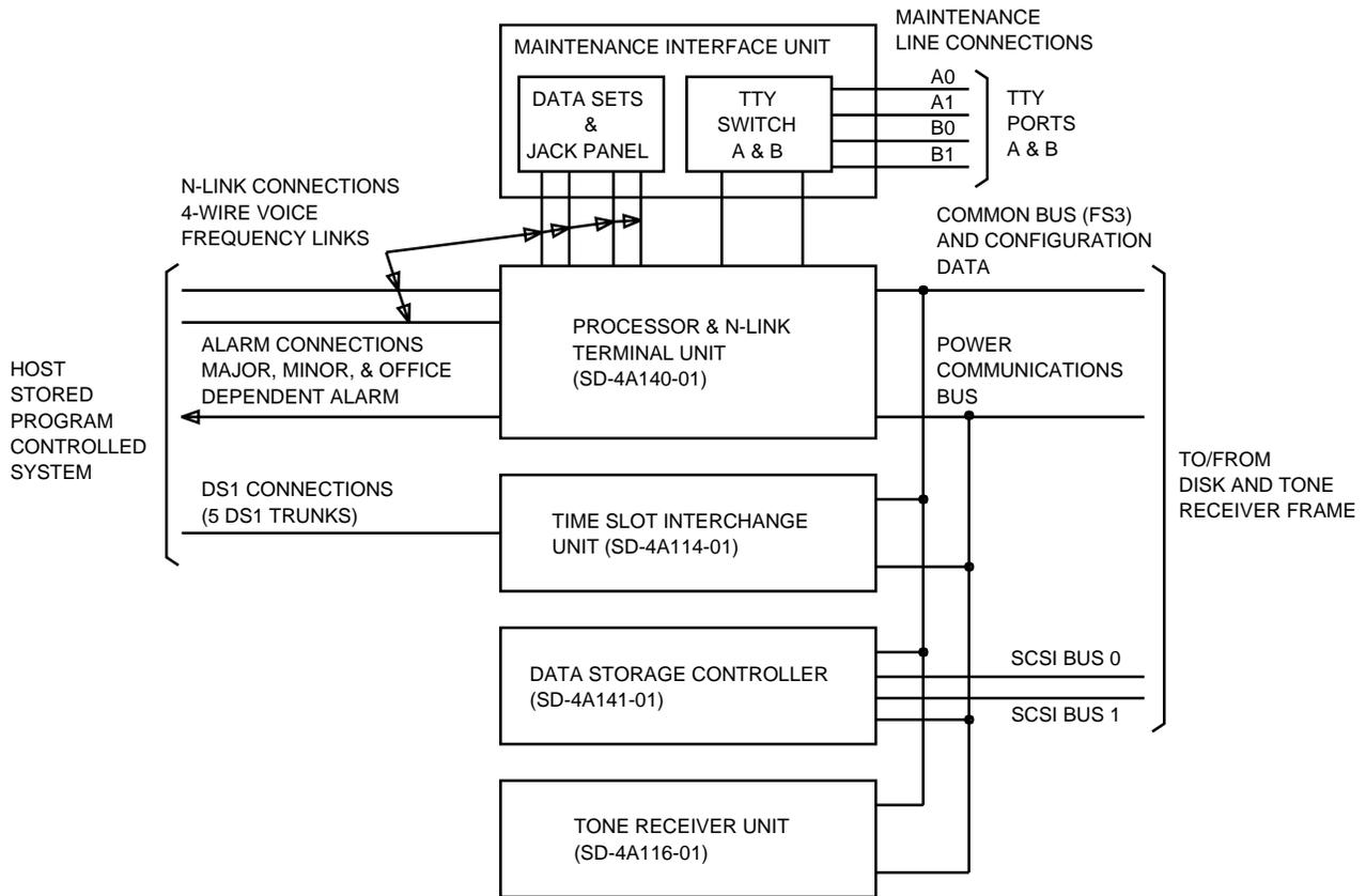
**Figure 38. Network Services Frame — Functional Block Diagram - SD4A139-01, J4A017G-1**
