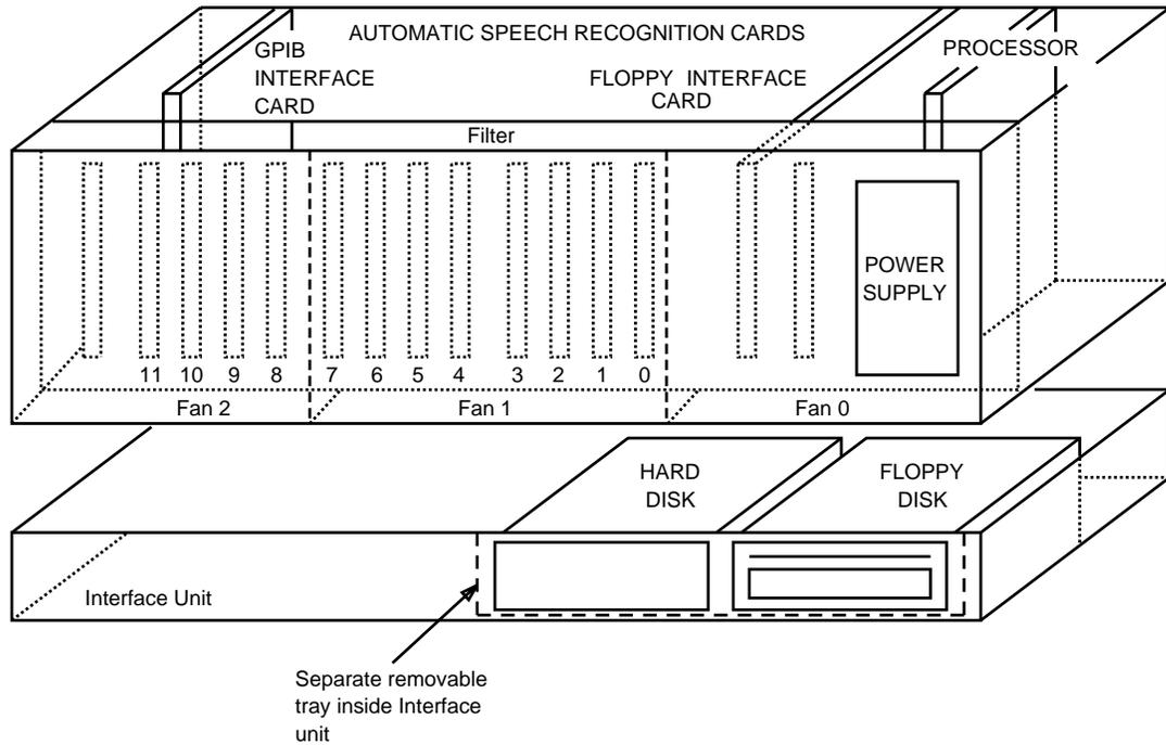
**Figure 28. ASR Unit and ASR Interface Unit**
