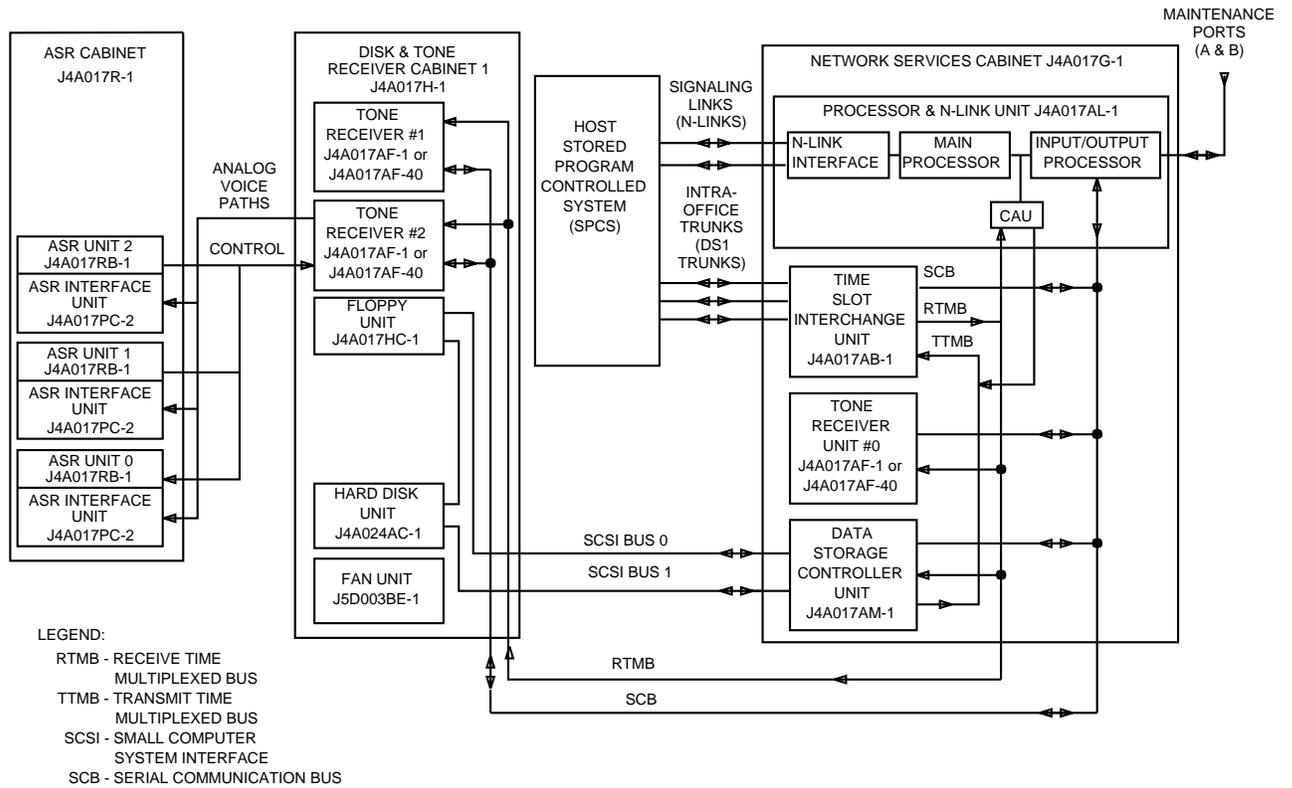
Figure 29. Direct Services Dialing Capability NSCX — Functional Block Diagram DSD8 or Later Generic
