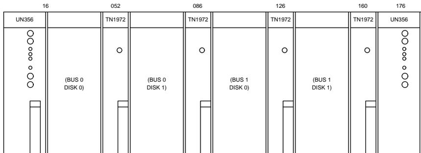
Figure 22. Hard Disk Unit J4A024AC-1
