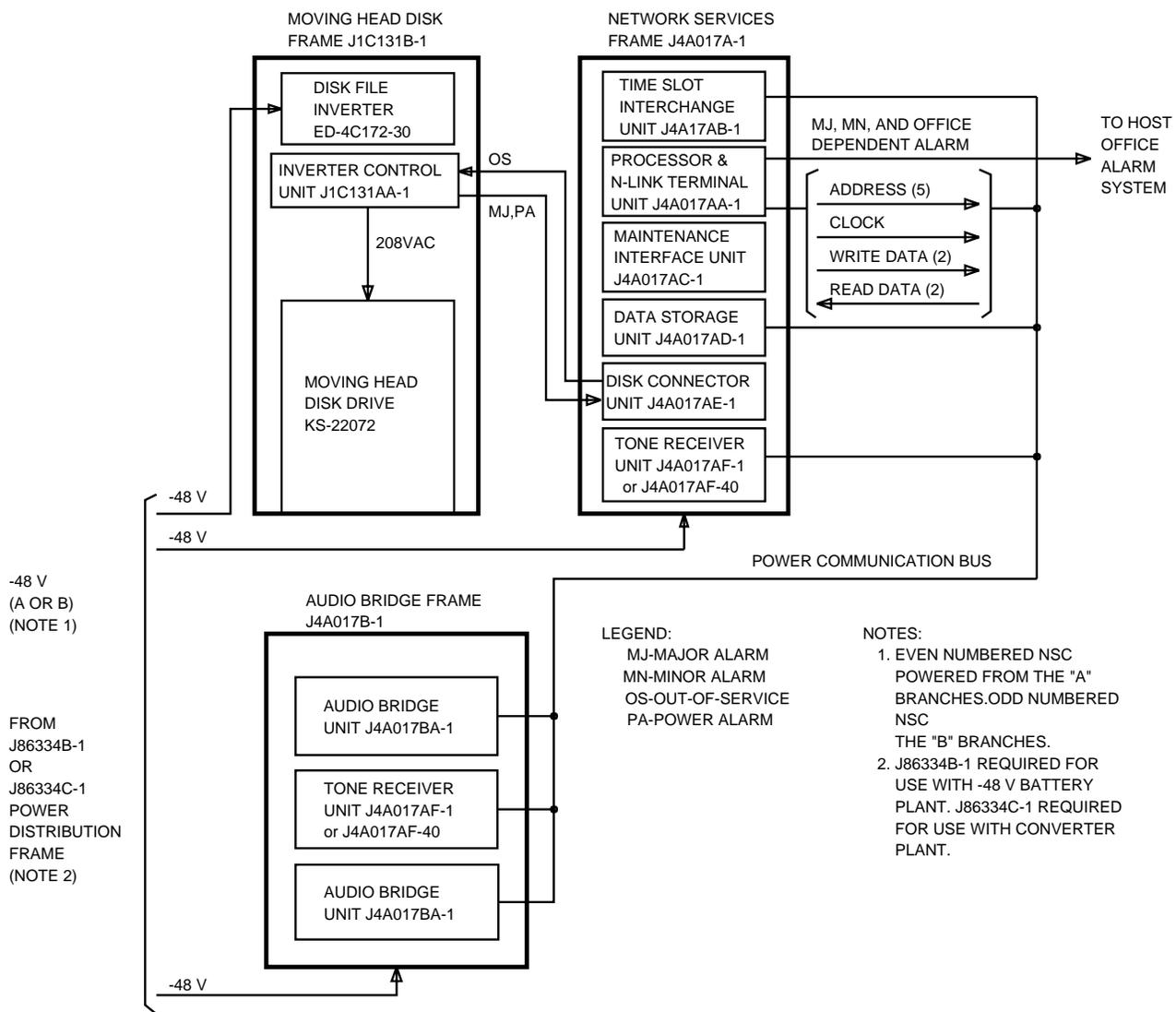
**Figure 42. Voice-Only or Voice Analog Graphics Teleconferencing Network Services Complex Power Distribution and Alarms — Functional Block Diagram**
