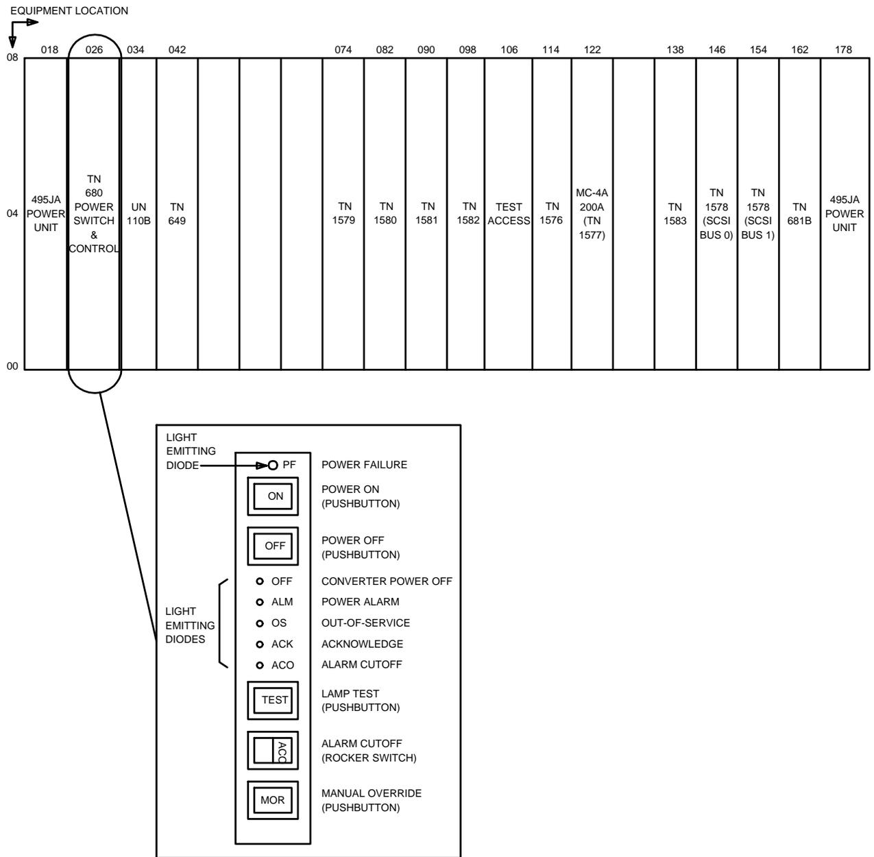
Figure 18. Data Storage Controller Unit J4A017AM-1 — Equipment Identification
