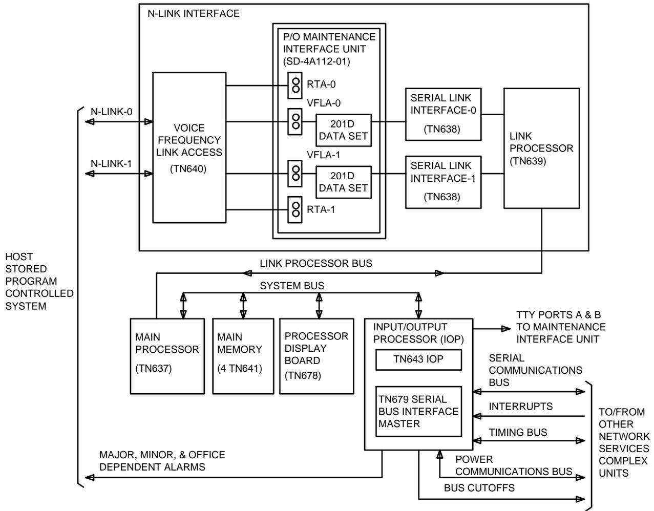
Figure 32. Processor and N-Link Terminal Unit — Functional Block Diagram (SD-4A113-01)
