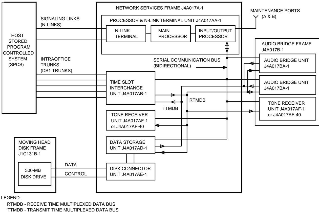
**Figure 30. Voice-Only or Voice and Analog Graphics Teleconferencing Network Services Complex — Functional Block Diagram**
