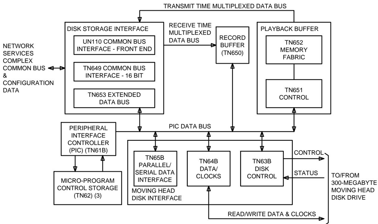
Figure 34. Data Storage Unit — Functional Block Diagram (SD-4A115-01)
