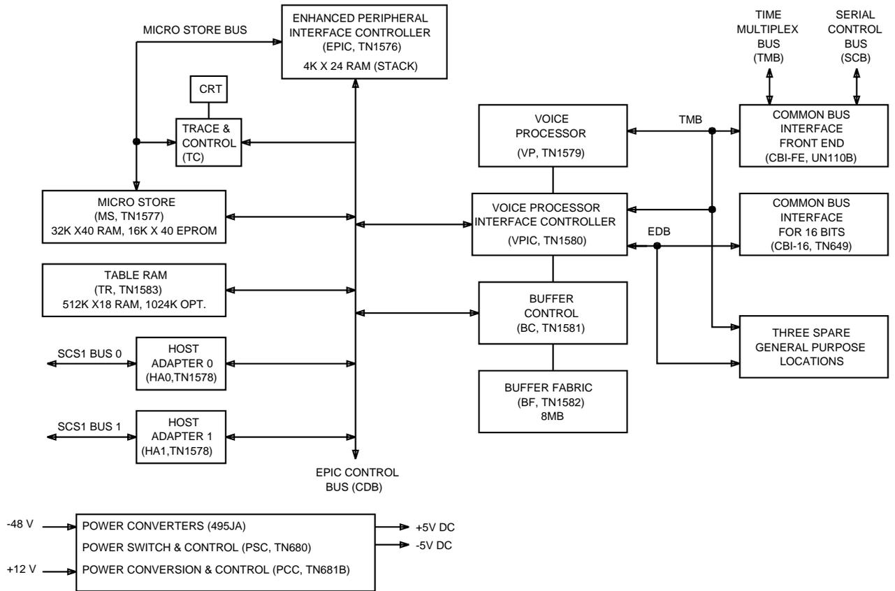
Figure 41. Data Storage Controller Unit SD4A141-01 — Functional Block Diagram
