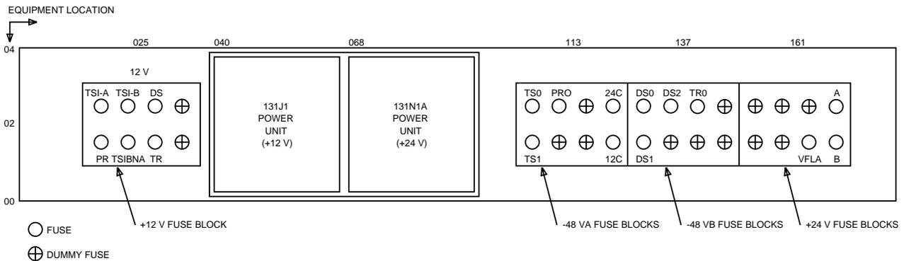
**Figure 10. Fuse Panel J4A017AG-1 — Equipment Identification**
