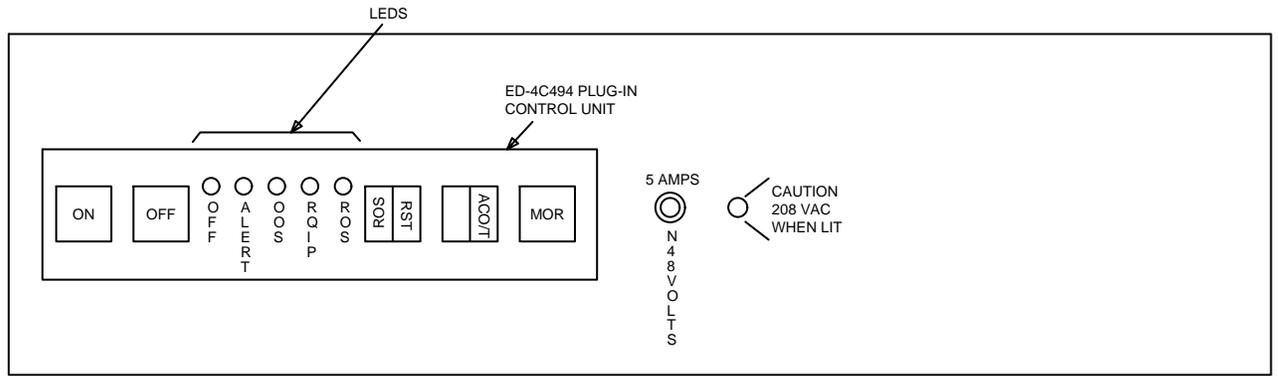
**Figure 25. Inverter Control Unit J1C131AA-1 — Equipment Identification**
