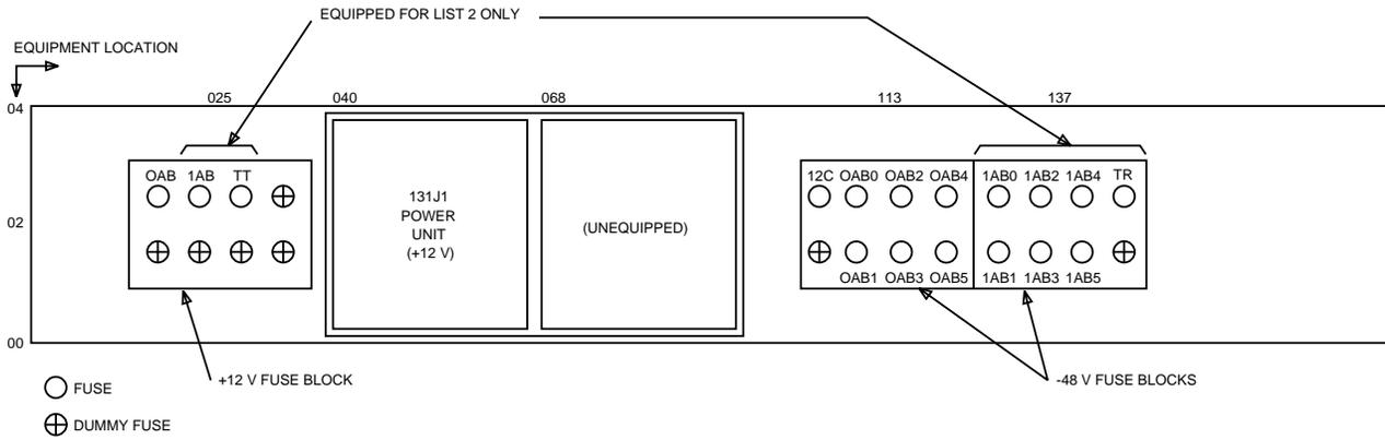
**Figure 13. Fuse Panel J4A017BB-1 — Equipment Identification**
