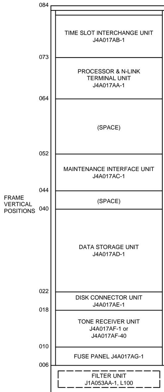
Figure 4. Network Services Frame (J4A017A-1) — Equipment Identification
