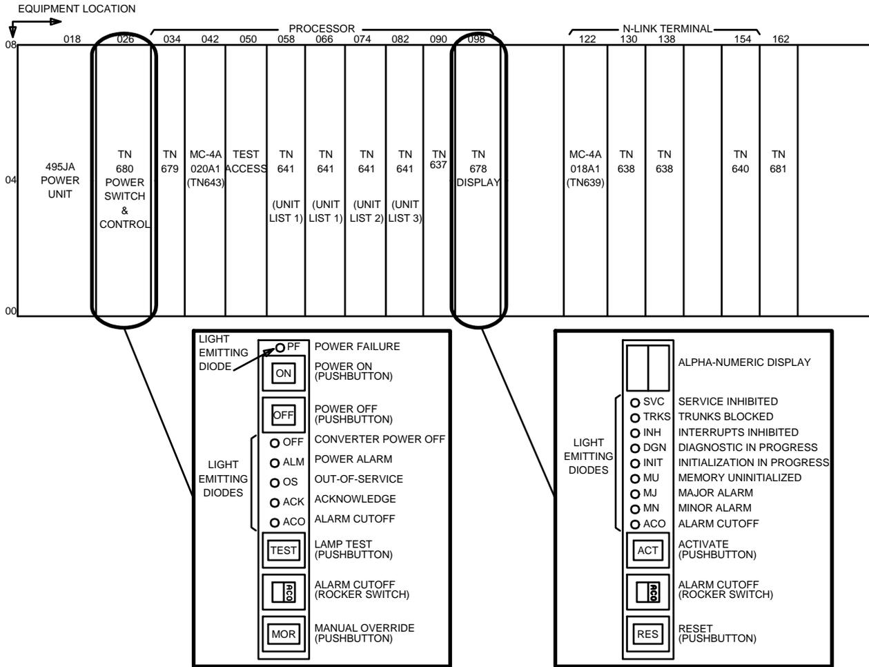
Figure 5. Processor and N-Link Terminal Unit J4A017AA-1 — Equipment Identification
