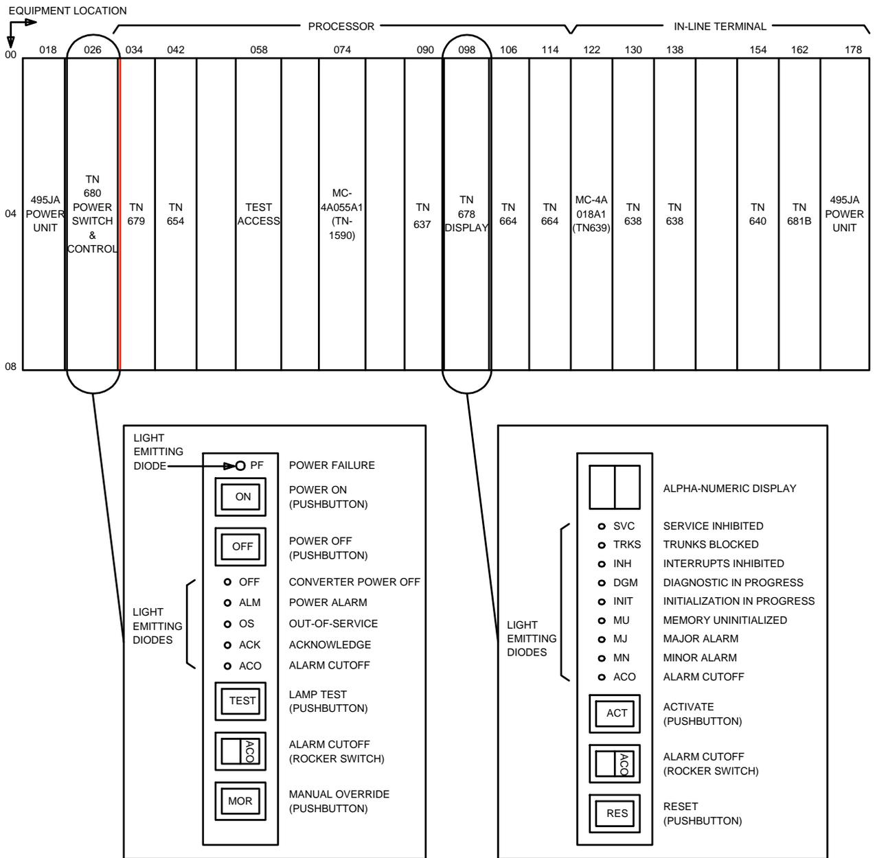
Figure 17. Processor and N-link Terminal Unit J4A017AL-1 — Equipment Identification
