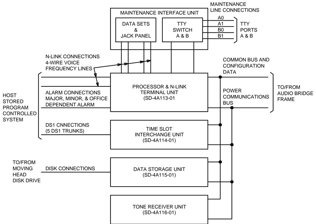
Figure 31. Network Services Frame — Functional Block Diagram (SD-4A112-01 [J4A017A-1])
