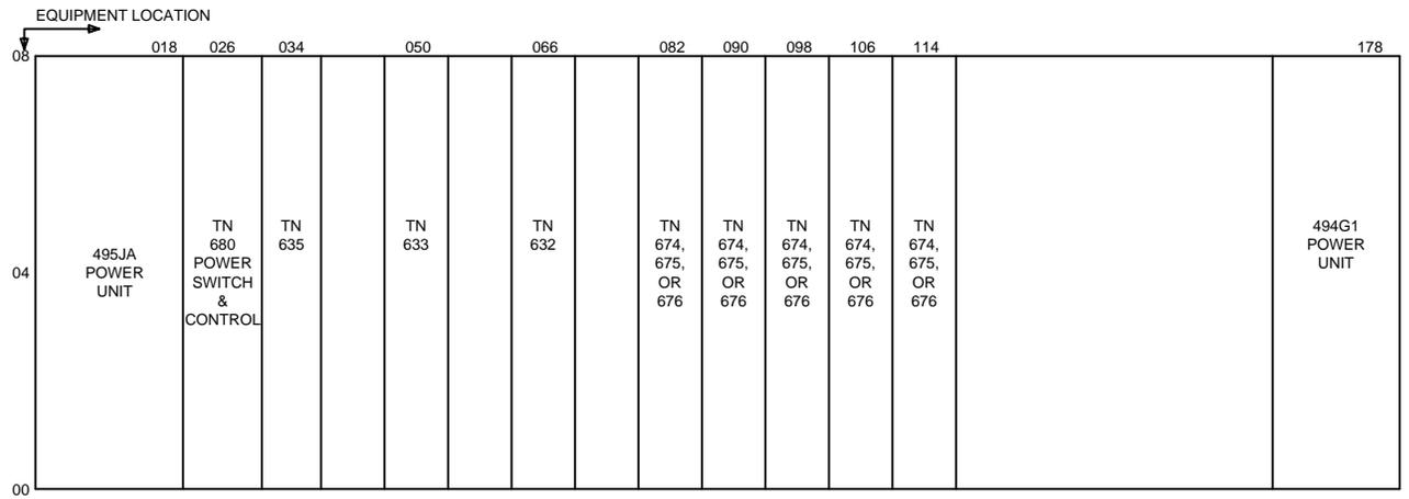
Figure 6. Time Slot Interchange Unit—Equipment Identification
