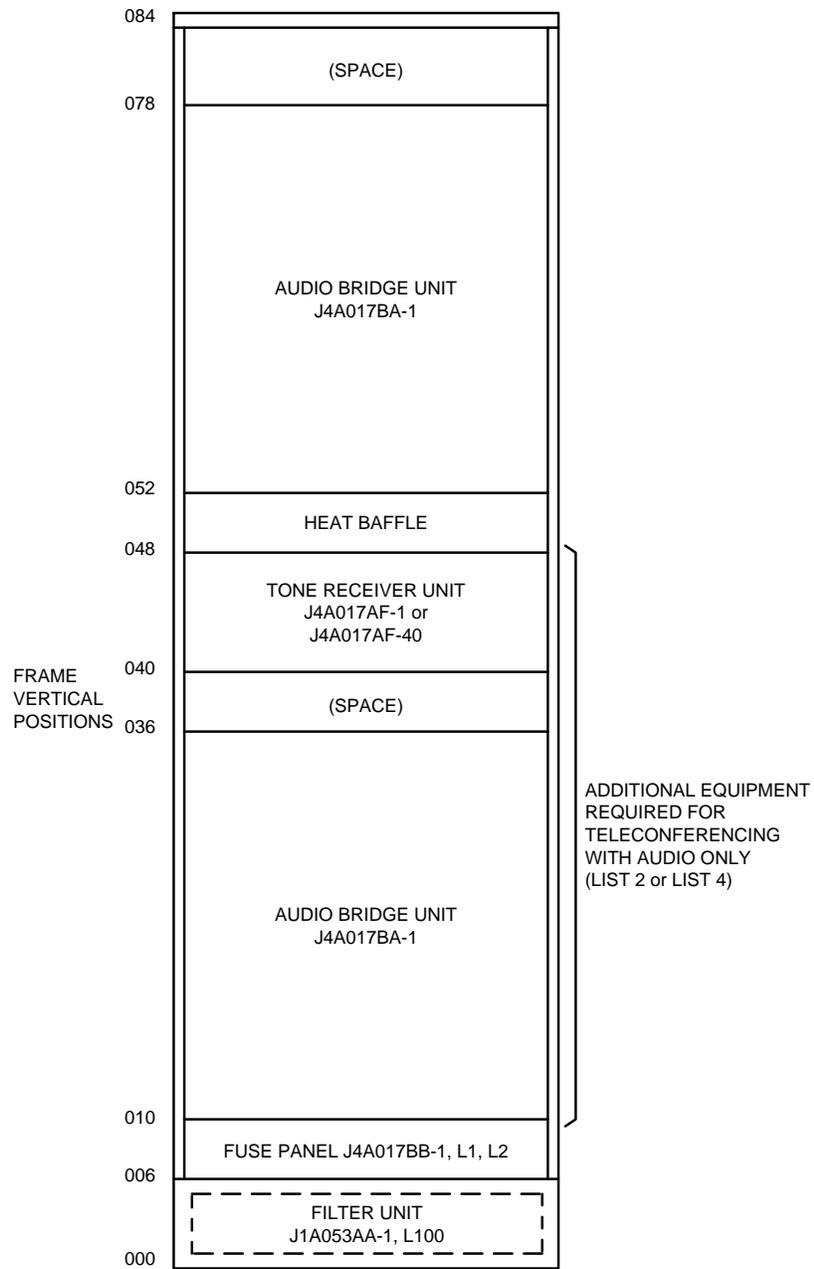
Figure 11. Audio Bridge Frame J4A017B-1 — Equipment Identification
