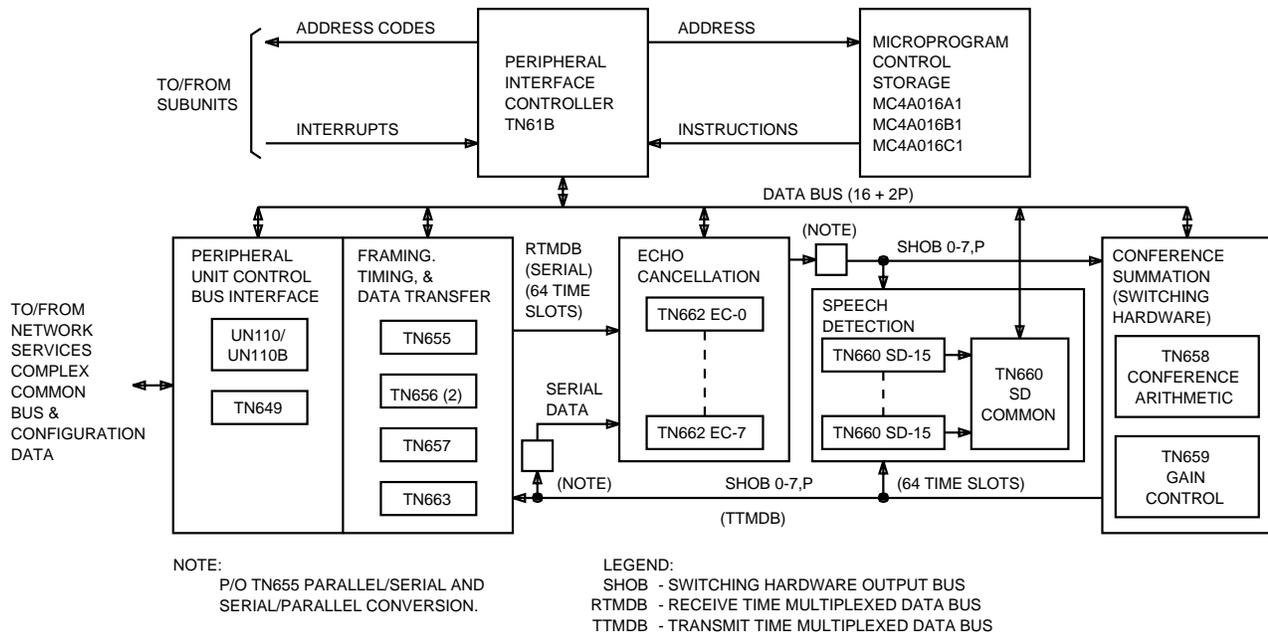
Figure 37. Audio Bridge Unit — Functional Block Diagram (SD4A118-01)
