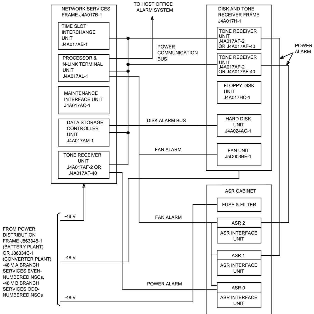
**Figure 43. Direct Services Dialing Capability NSCX Power Distribution and Alarms — Functional Block Diagram DSD8 or Later Generic**
