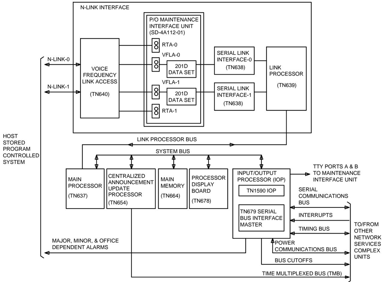
Figure 39. Processor and N-link Terminal Unit - SD4A140-01, J4A017AL-1 — Functional Block Diagram
