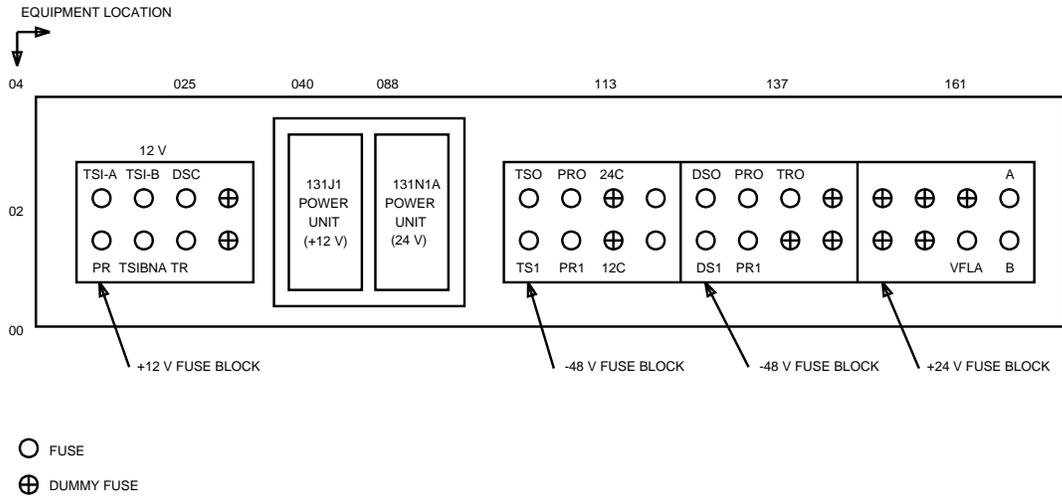
**Figure 19. Fuse Panel J4A017GA-1 — Equipment Identification**
