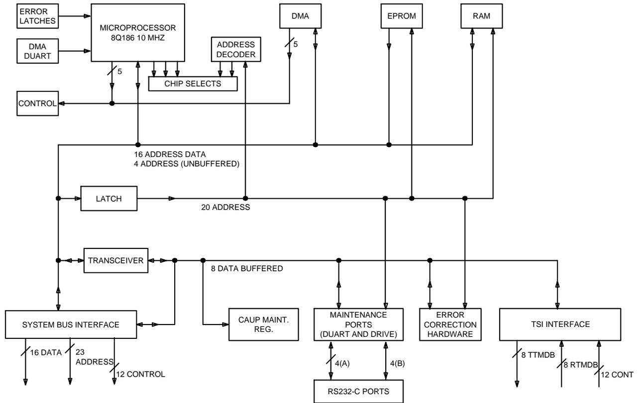
**Figure 40. Centralized Announcement Update Processor — Functional Block Diagram**
