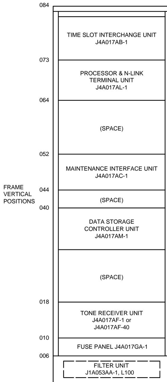
Figure 16. Network Services Frame J4A017G-1 — Equipment Identification
