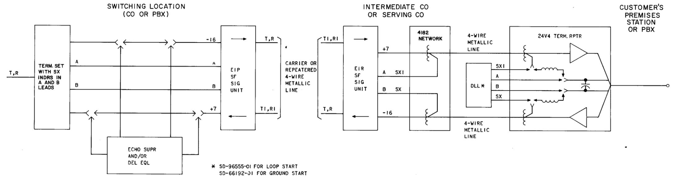
Fig. 5—Single Frequency Signaling Loop Start or Ground Start Using EIP-EIR
