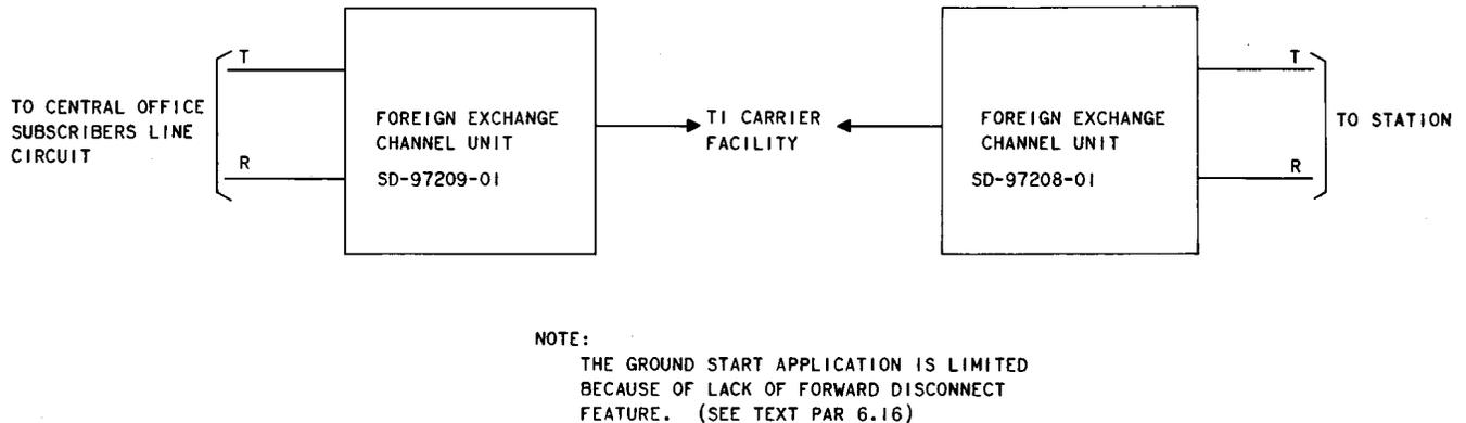
**Fig. 9—T1 Carrier Foreign Exchange Channel Units Loop Start and Ground Start**
