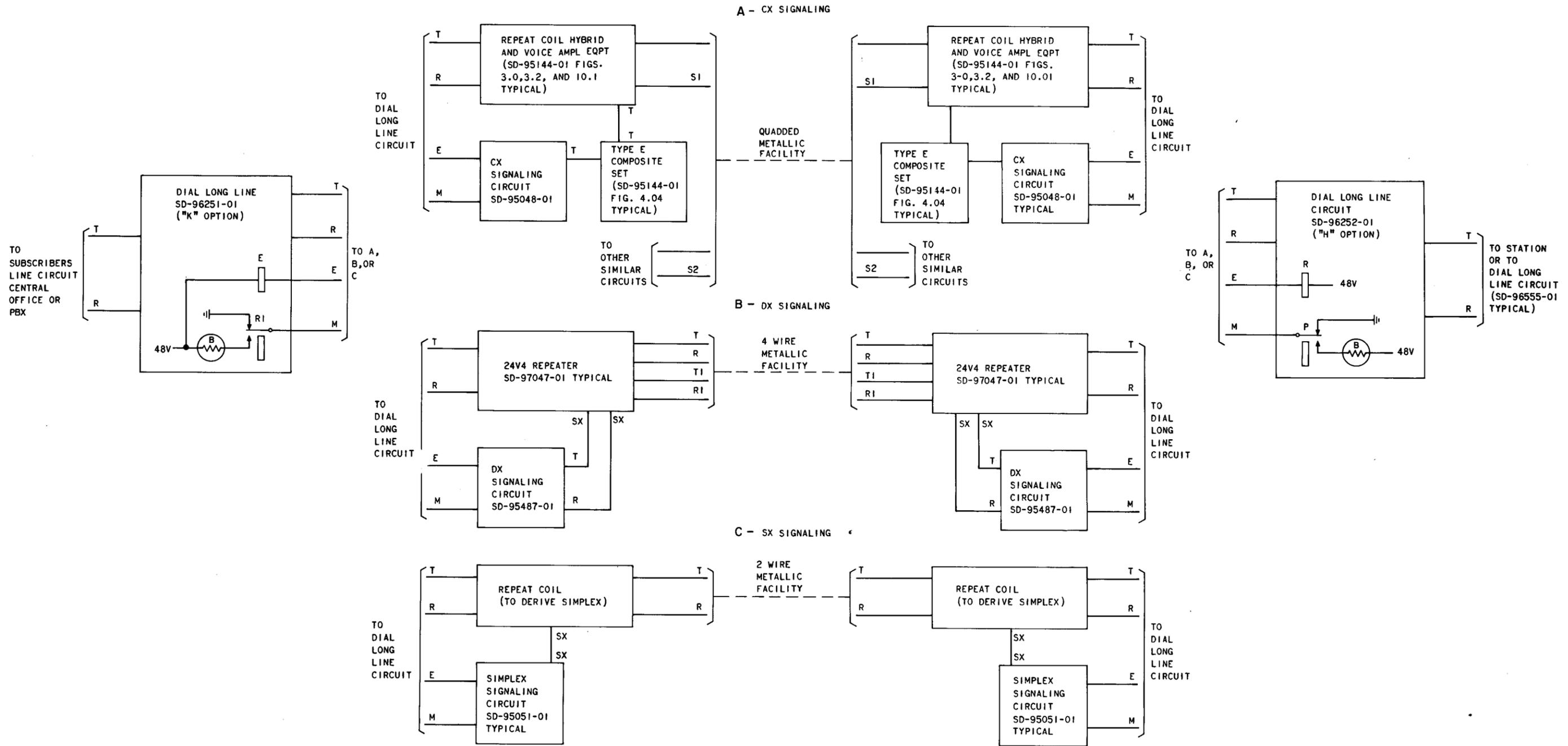
Fig. 3—CX, DX, and SX Signaling on Metallic Facilities Loop Start
