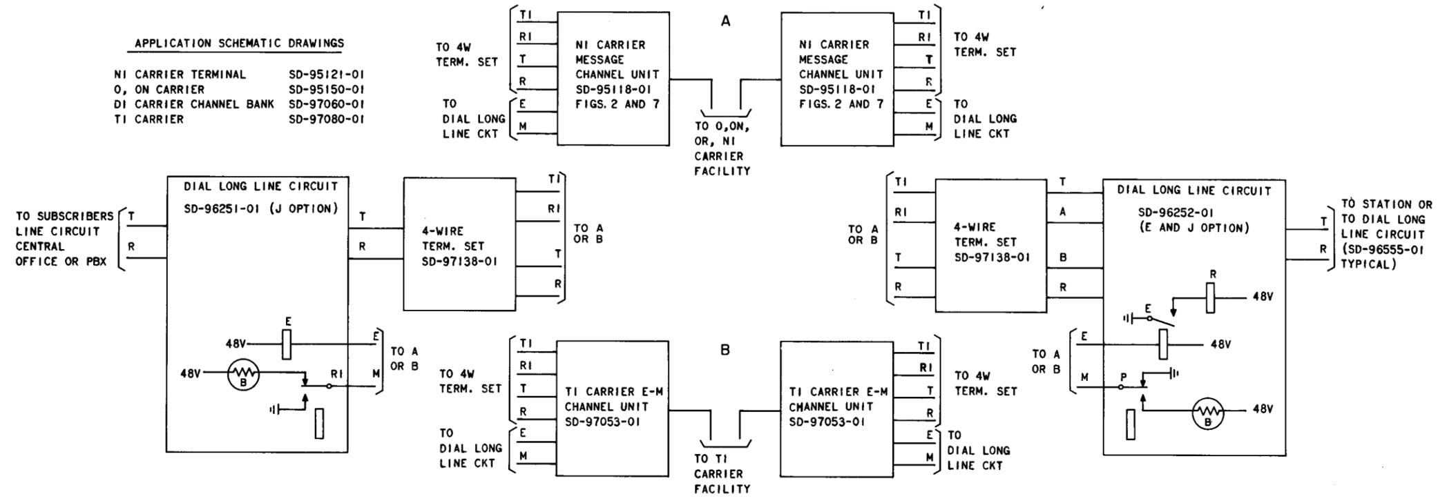
Fig. 4—Out-of-Band Signaling O, ON, NI, and T1 Carrier Systems Loop Start
