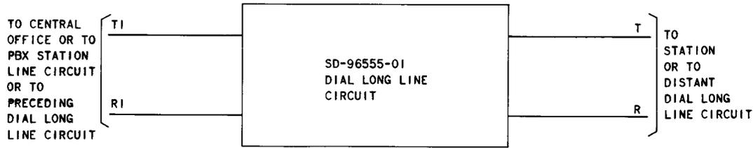
Fig. 1—Metallic Loop Signaling Loop Start
