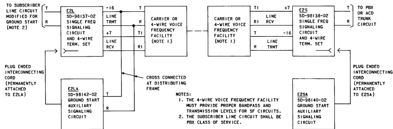
Fig. 7—Single Frequency Signaling Ground Start Using E2L-E2S and E2LA-E2SA
