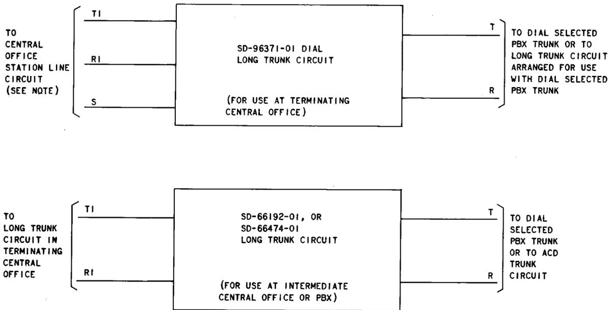
**NOTE:** THIS CIRCUIT IS TO BE CONNECTED TO AN ORDINARY SUBSCRIBERS LINE CIRCUIT IN WHICH THE LINE RELAY OPERATES FROM A BRIDGE ACROSS THE "TI" AND "RI" LEADS. (THE SLEEVE LEAD PROVIDES THE EQUIVALENT OF GROUND START TYPE OPERATION).
