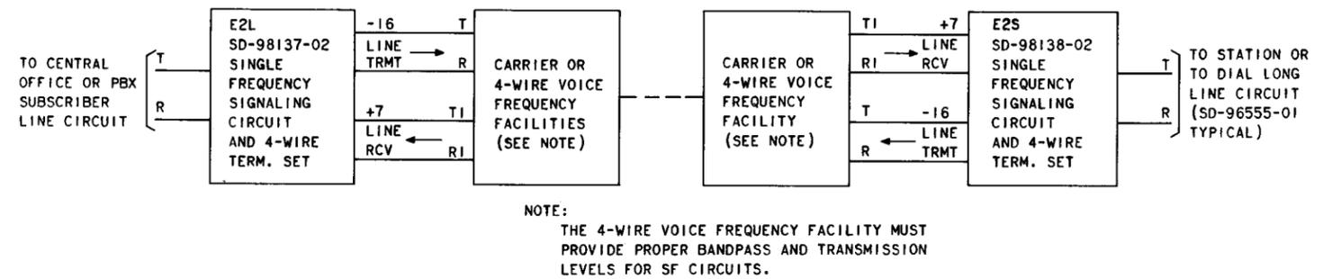
Fig. 6—Single Frequency Signaling Loop Start Using E2L-E2S
