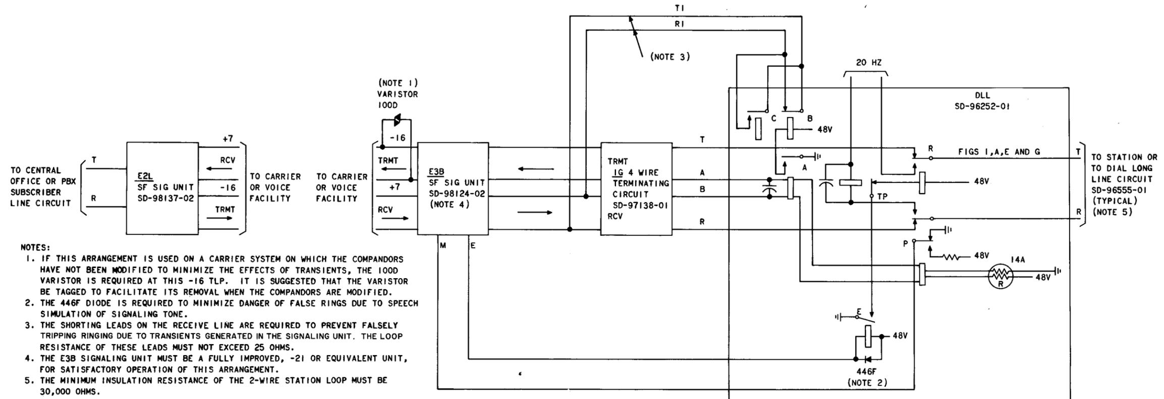
Fig. 8—Single Frequency Signaling Loop Start Using E2L, E3B, and DLL SD-96252-01
