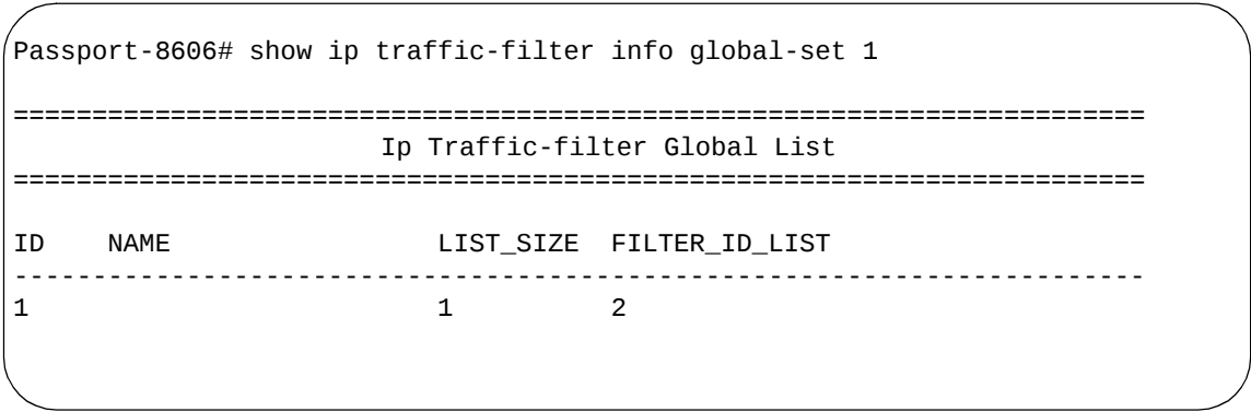
Figure 75 show ip traffic-filter info global-set command output
