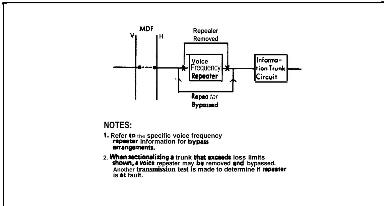
Exhibit 12 – Trunk Retesting With Voice Frequency Repeater Removed
