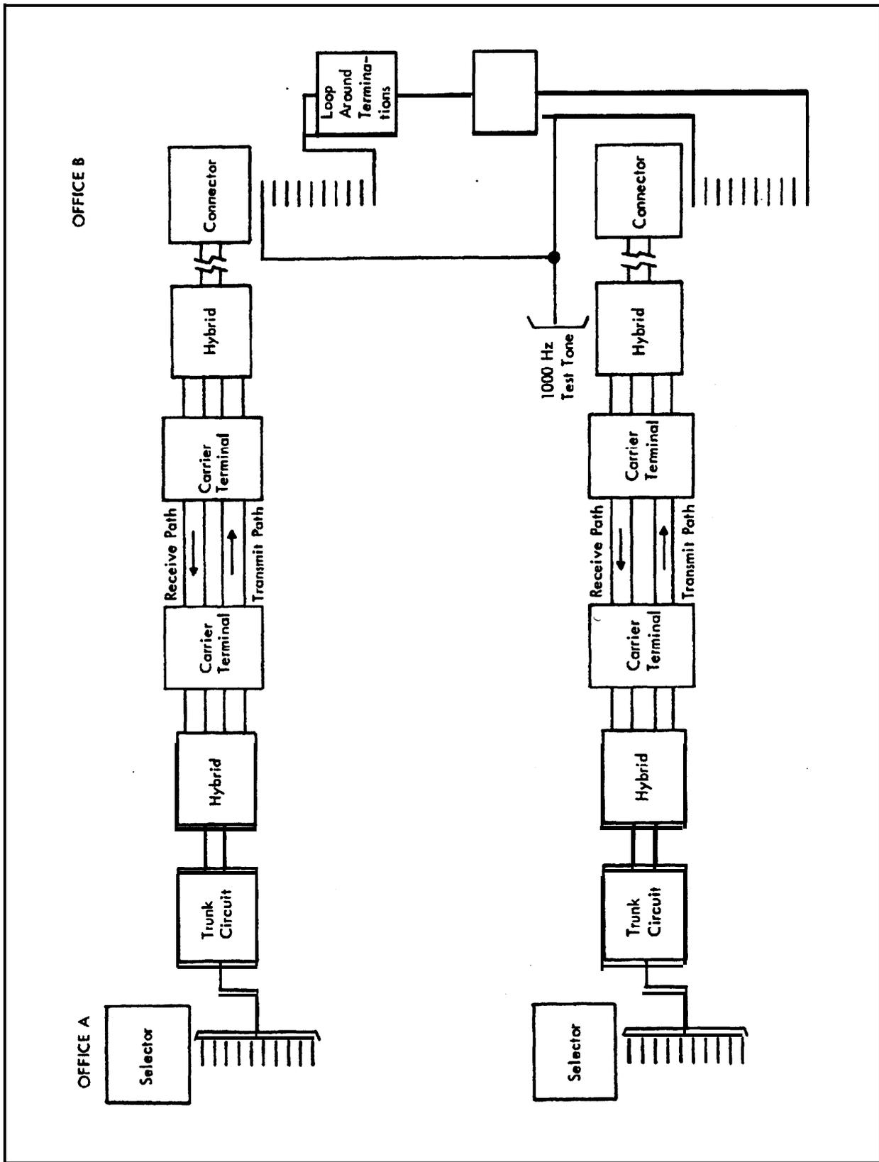
Exhibit 14 - Loop-Around Transmission Testing Showing Selector Access to Loops
