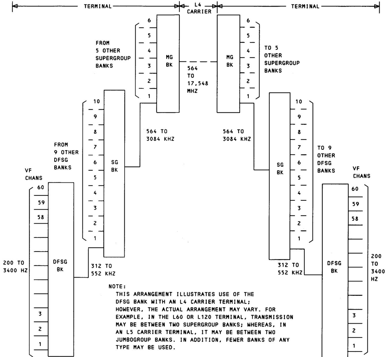
Fig. 2—Typical Function of the DFSG Bank in the L-Type Terminal
