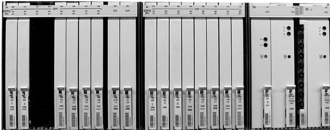
Figure 1-17. DSPU Circuit Pack Locations
