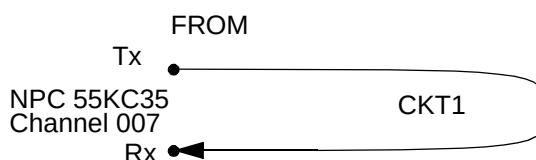
Figure 9-6. Sample Half-Duplex Loopback Circuit
