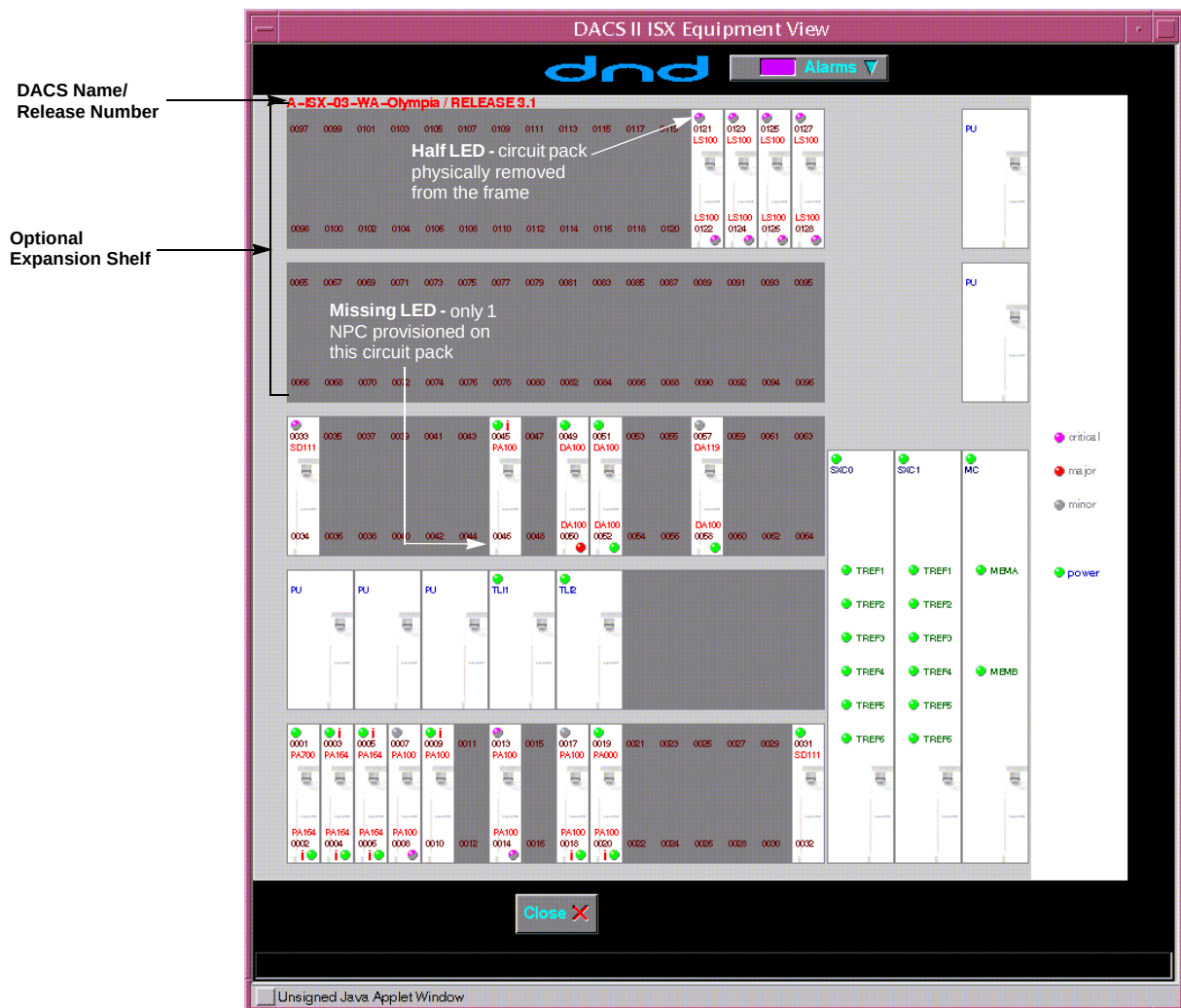
Figure 13-18. DACS II ISX Equipment View
