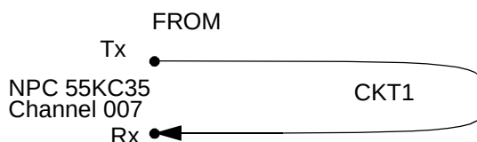
Figure 9-6. Sample Half-Duplex Loopback Circuit
