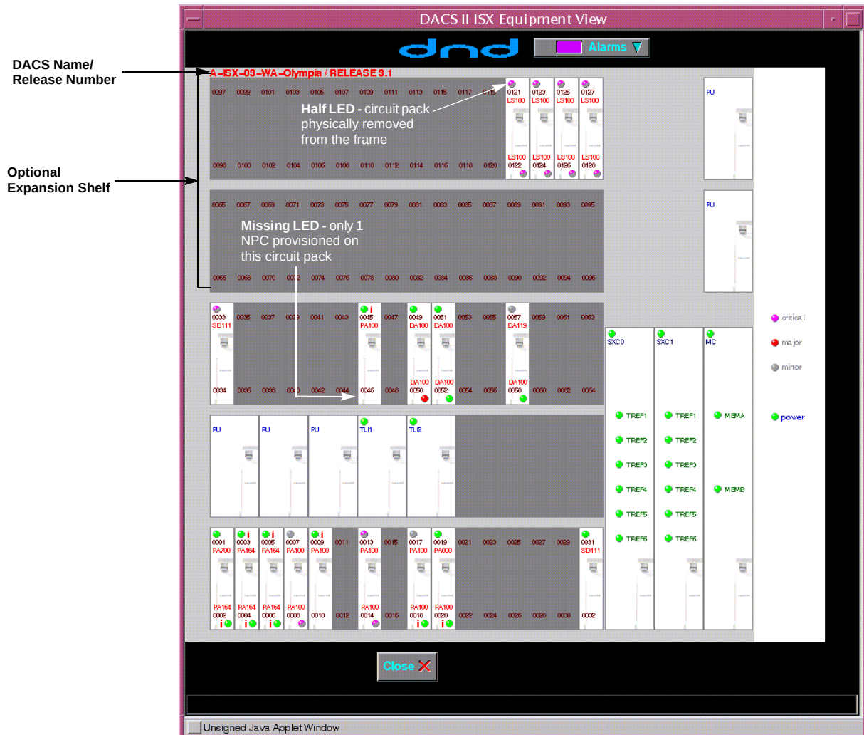
Figure 13-18. DACS II ISX Equipment View
