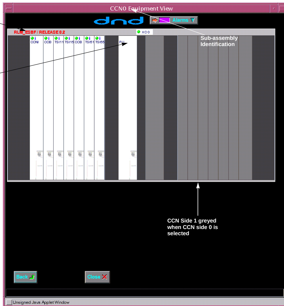
Figure 13-12. DACS II Equipment View - DACS II E/SBF CCN
