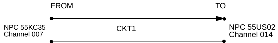
Figure 9-3. Sample Half-duplex Circuit
