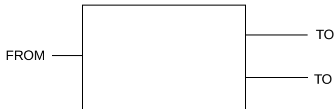
Figure 9-8. Ideal Broadcast Circuit
